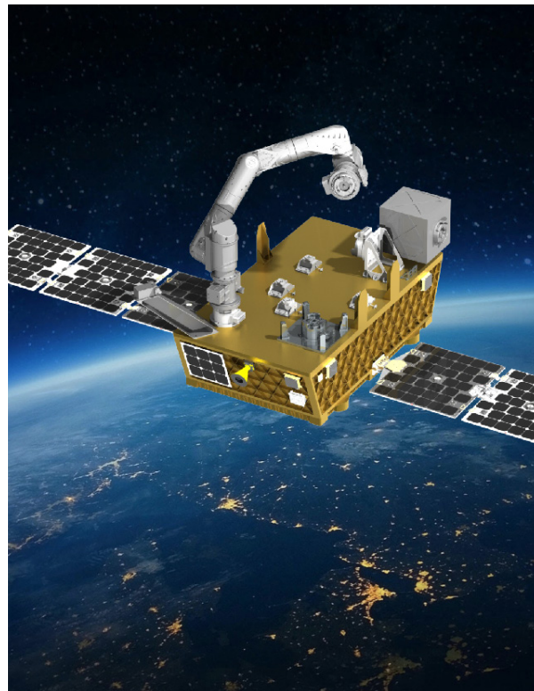
The Fly Foundational Robots (FFR) spacecraft with robotic arm payload envisioned in orbit, image provided by Motiv Space Systems.
