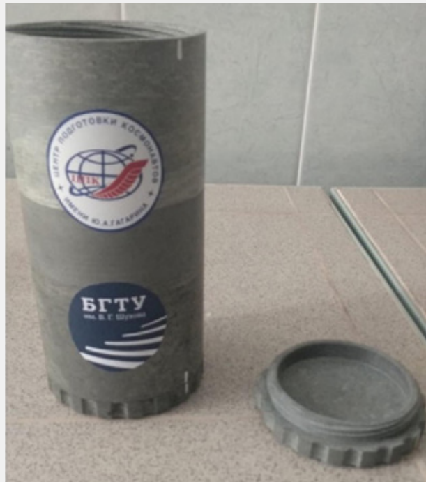
Figure 21. Photo of the polymer composite fitted with radiation detectors. Image adapted from Cherkashina, Advances in Space Research .
