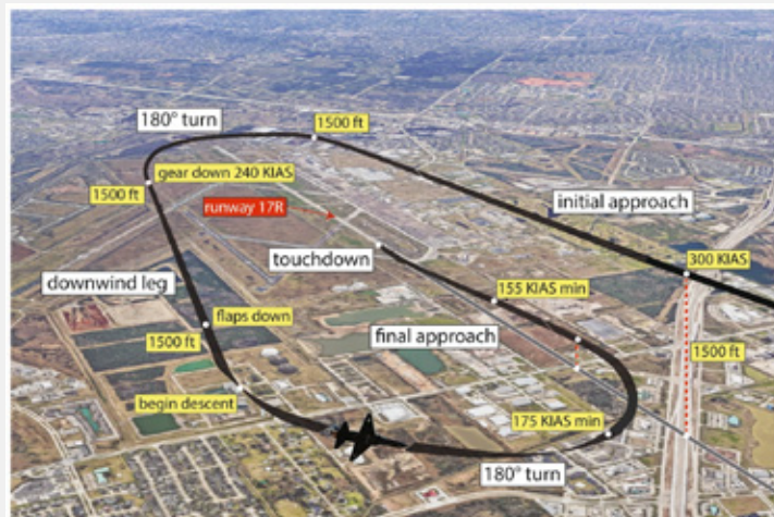
Figure 20. Flight path used in a T-38 landing simulation. Performance was evaluated using parameters such as touchdown location and vertical speed. Image adapted from Moore, Scientific Reports.
