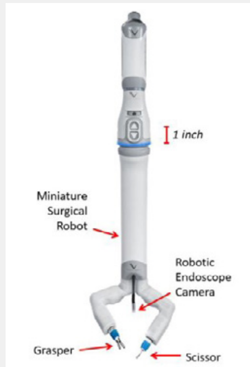
Figure 28. Image of the miniature surgical robot spaceMIRA used aboard the space station. Image adopted from Wagner, AIAA AVIATION FORUM AND ASCEND 2025.
