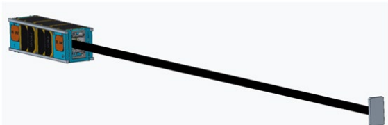
Figure 6.5: GPX-2 CAD image with gravity gradient boom deployed. Credit: NASA.
