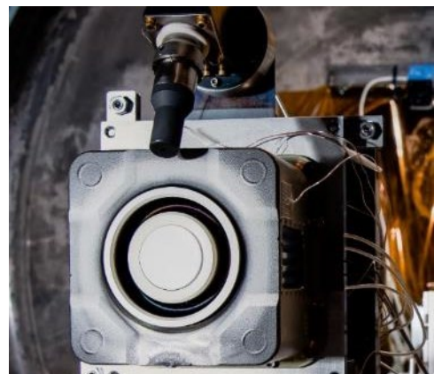
Figure 4.41: BHT-600 Installed in NASA GRC Vacuum Test Facility. Credit: Busek Co.
