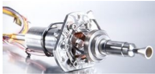
Figure 4.3: ECAPS HPGP thruster. Credit: Bradford ECAPS.
