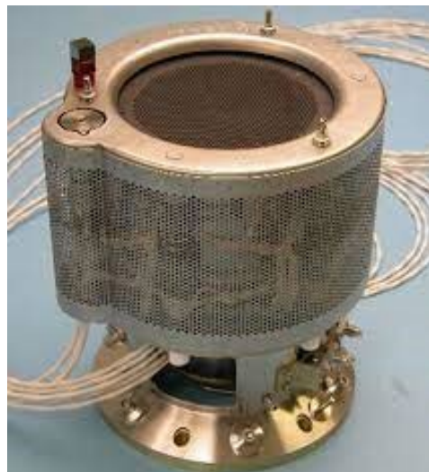
Figure 4.27: T5 gridded-ion thruster for GOCE mission. Credit: QinetiQ.
