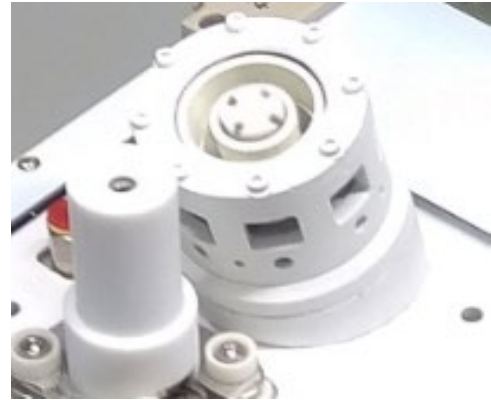
Figure 4.35: spaceware-nano thruster. Credit: Exotrail.
