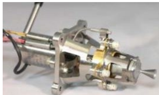
Figure 4.5: GR1 thruster. Credit: Aerojet.
