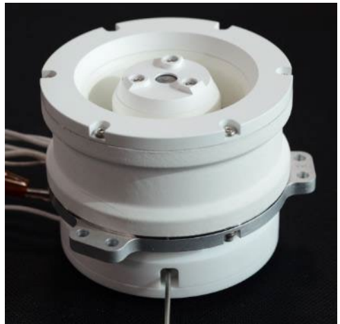
Figure 4.37: Halo thruster. Credit: ExoTerra Resource.
