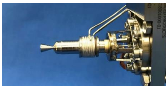
Figure 4.7: Rubicon 0.1N ASCENT thruster. Credit: NASA MSFC.
