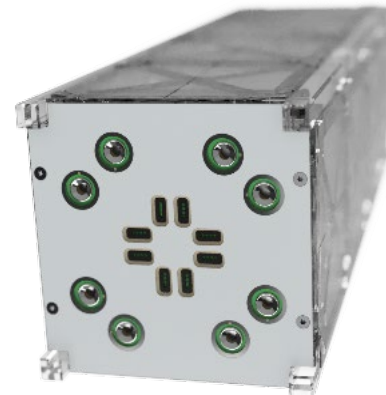
Figure 4.24: Eight NanoFEEP thrusters integrated on 3U-Cubesat bus. Credit: Morpheus Space.
