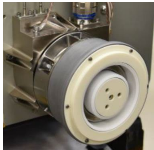
Figure 4.42: NGHT-1X Engineering Model Hall-Effect Thruster. Credit: Northrop Grumman.
