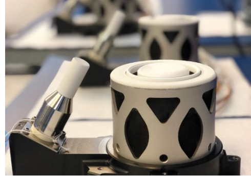
Figure 4.40: BHT-350 Flight Units. Credit: Busek Co.
