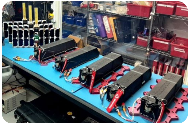
Figure 2.4: Alba Orbital Integration of PocketQubes into the Deployers. Credit: Alba Orbital.
