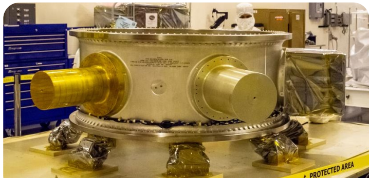
Figure 2.9: LandSat-9 ESPA Ring populated with payloads and mass ballasts. Credit: NASA/Randy Beaudoin.
