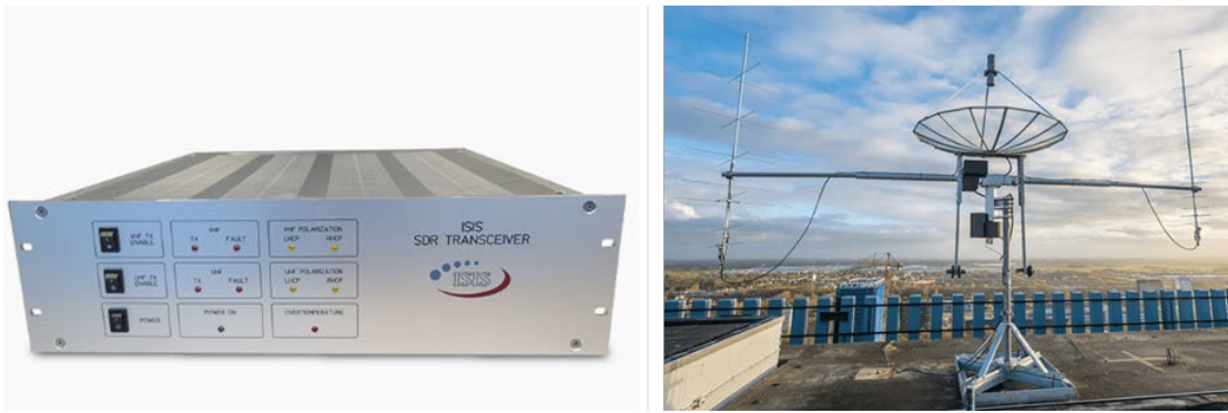
Figure 11.22: (left) ISIS ground station hardware, transceiver rack and tracking antenna (right). Credit: ISISPACE.
