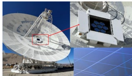
Figure 11.36: JPL's DSS-13, a 34m RF antenna, showing a 1.3-meter optical aperture in its center. Credit: NASA JPL.
