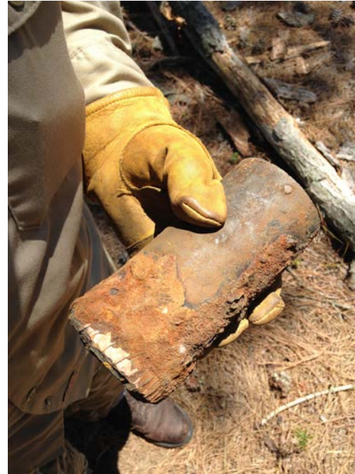
Photograph 16: 2.75 inch MD cylinder with rotating bands found along transect BB-AT05 on south side of Boat Basin.
