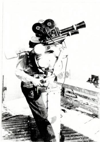
Modified Mk 51 Director Used As Phototheodolite on Sea Stand
