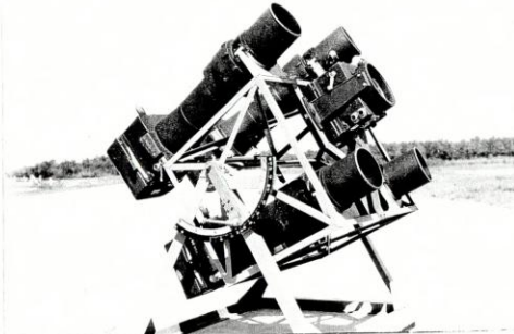
F-56 Camera Cluster Now Used at Bullseye for Dove Project
