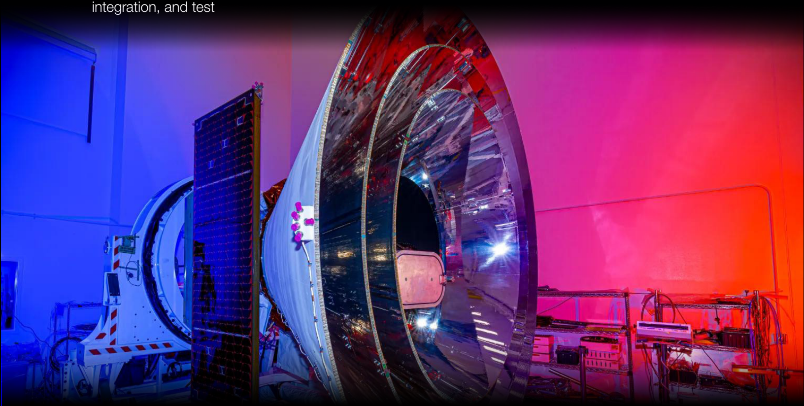
Image Caption: The SPHEREx space observatory was photographed in November 2024 after completing environmental testing. The spacecraft was launched on March 11, 2025. The spacecraft’s three large concentric cones help direct heat and light away from the telescope and other components, keeping them cool. Credit: NASA/JPL-Caltech/BAE Systems
