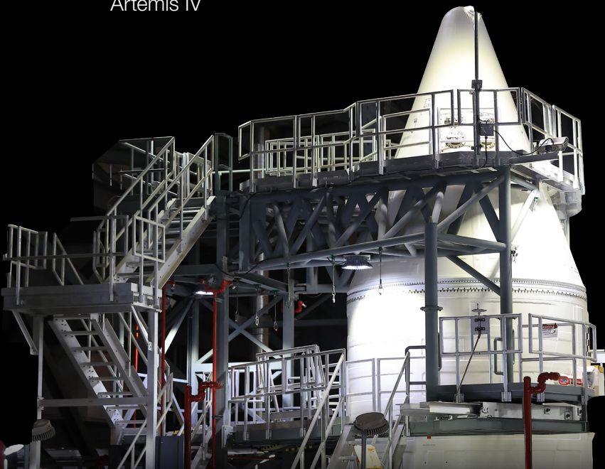
Image Caption: Engineers complete stacking operations on the twin Space Launch System (SLS) solid rocket boosters for Artemis II by integrating the nose cones atop the forward assemblies inside the Vehicle Assembly Building’s High Bay 3 at NASA’s Kennedy Space Center in Florida on February 19, 2025. Credits: NASA/K. Shiflett
