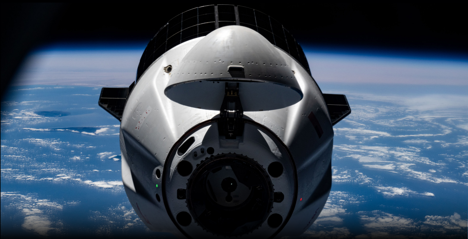
Image Caption: A SpaceX Dragon cargo spacecraft with its nosecone open approaches the International Space Station for an automated docking to the Harmony module’s forward port while carrying more than 5,000 pounds of science, supplies, and hardware for the CRS-33 mission. Both vehicles are flying 261 miles above the Atlantic Ocean south of the Azores at the moment captured. Credits: NASA/JSC
