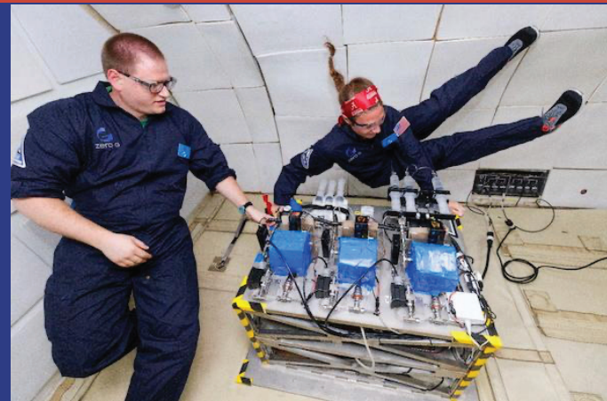
Bill Doig (left) and Brianna Warrenfeltz (right) operating the Teledyne EDR fuel cell water separator experiment during a reduced-gravity parabola on the first day of testing.
