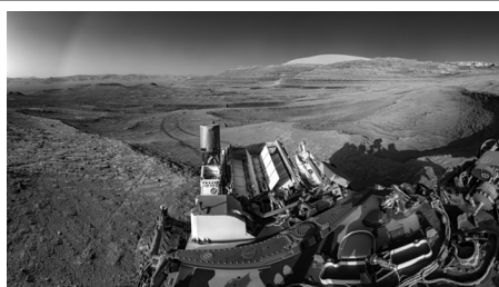
This view of tracks trailing NASA's Curiosity was captured July 26, 2025, as the rover simultaneously relayed data to a Mars orbiter. Combining tasks like this more efficiently uses energy generated by Curiosity's nuclear power source, shown here, lined with rows of white fins at the back of the rover. Credit: NASA/JPL-Caltech
