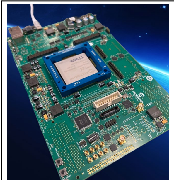
Pictured here is a production HPSC processor on a test board at Microchip facilities. This new, space-qualified commercial processor enables complex applications such as precision landing and autonomous robotics operations.
