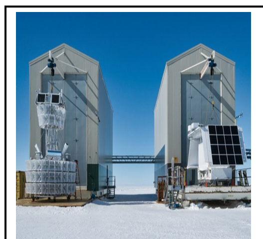
Astrophysics Balloon Payloads on the Ross Ice Shelf near McMurdo Station, Antarctica. On the left is the Pioneers Mission PUEO, a radio detector searching for impulsive radio signature that ultra high-energy neutrinos generate when they interact with the vast Antarctic ice, which serves as the detection volume. On the right is the General Antimatter Particle Spectrometer, which is searching for dark matter signatures by detecting antimatter in the cosmic radiation.
