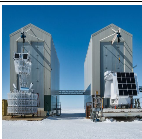
Astrophysics Balloon Payloads on the Ross Ice Shelf near McMurdo Station, Antarctica. On the left is the Pioneers Mission PUEO, a radio detector searching for impulsive radio signature that ultra high-energy neutrinos generate when they interact with the vast Antarctic ice, which serves as the detection volume. On the right is the General Antimatter Particle Spectrometer, which is searching for dark matter signatures by detecting antimatter in the cosmic radiation.
