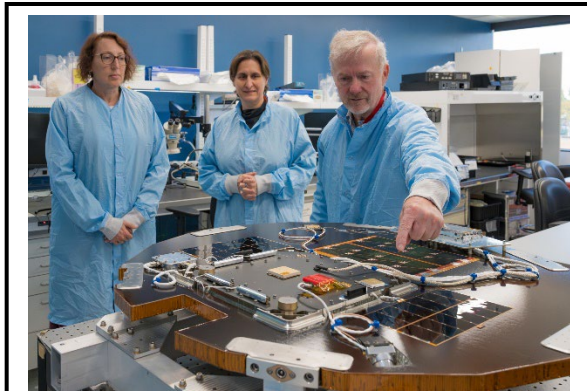
Team members from the Aerospace Corporation and NASA inspect a DiskSat spacecraft before it launched with three others in December 2025. DiskSat is a joint NASA and U. S. Space Force effort developed for small spacecraft missions needing higher power or larger apertures than CubeSats can provide.
