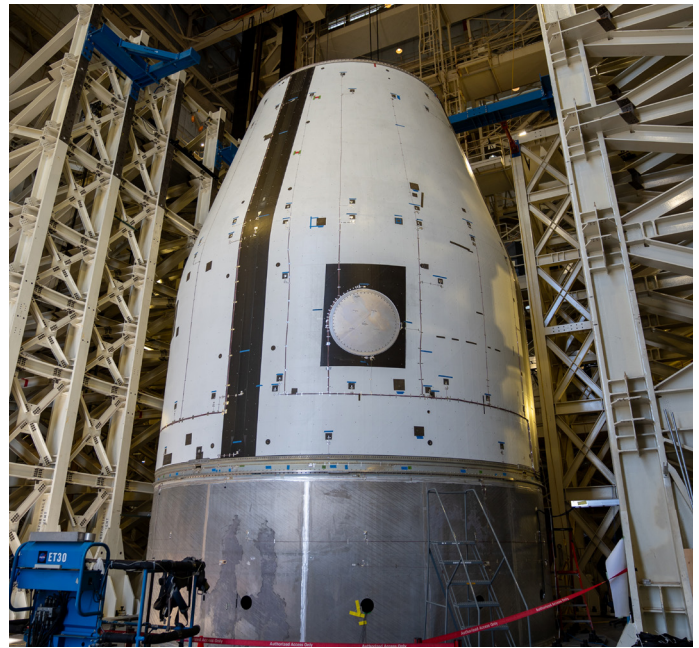
A test version of the SLS Block 1B universal stage adapter is moved into a test fixture at NASA's Marshall Space Flight Center in Huntsville, Alabama, to be subjected to simulated launch stresses. When Block 1B debuts on Artemis IV, the adapter will be capable of co-manifested payloads up to 10 metric tons (22,046 lbs.) and more than 10,000 cubic feet (283 cubic meters).
