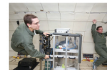
In 2011, NASA tested the RFMG in microgravity on parabolic flights supported by Flight Opportunities. Credits: Devin Bolot
