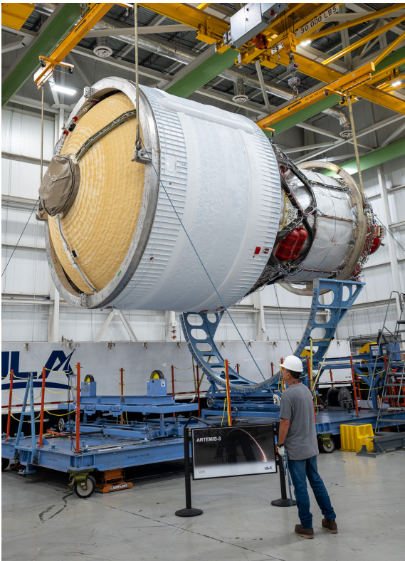
The interim cryogenic propulsion stage (ICPS), a modified United Launch Alliance Delta Cryogenic Second Stage, provides 24,750 lbs. of thrust for in-space propulsion for the Block 1 crew and cargo vehicles.
