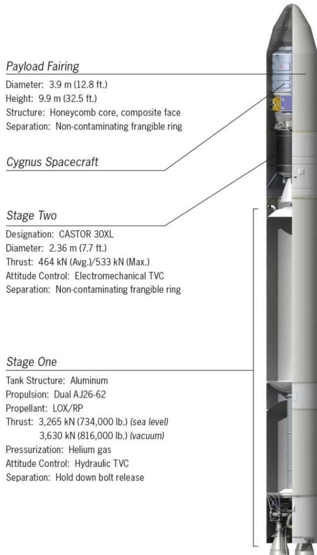
From its launch site at Wallops Island, Virginia, Antares is capable of supporting mid-inclination and polar orbiting spacecraft weighing up to approximately 13,500 lb. (6123 kg) and 5,500 lb. (2495 kg), respectively.
