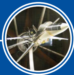
Forced Oscillation System
