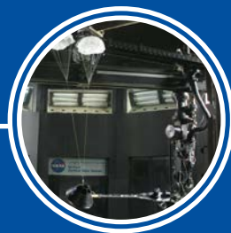
Rotary Balance System
