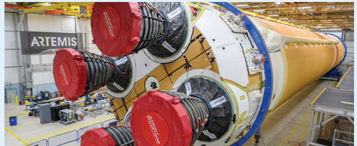
The Artemis II RS-25 engines were installed in the core stage during assembly at NASA's Michoud Assembly Facility in New Orleans.
