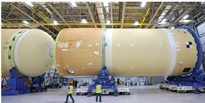
Workers at NASA's Michoud Assembly Facility in New Orleans are shown here preparing to join the core stage liquid hydrogen tank (left) to the core stage forward assembly (right) comprising the forward skirt, liquid oxygen tank, and intertank.
