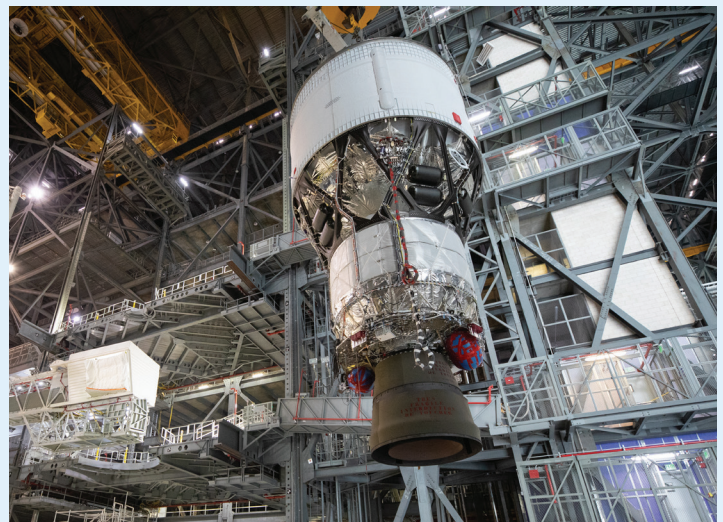
The four-story Artemis II interim cryogenic propulsion stage is seen here lifted for stacking on SLS to help send Orion to the Moon.
