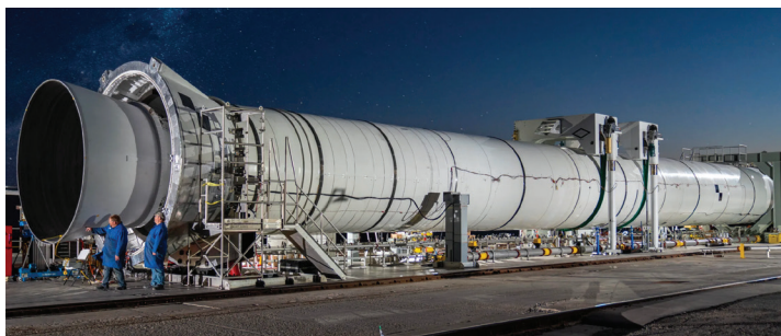
This image shows a close-up of the Flight Support Booster-2 solid rocket motor, poised for a full-scale ground test at Northrop Grumman's Utah test facility.
