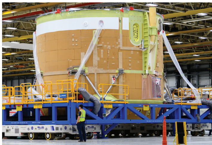
Workers are seen here moving the Artemis II core stage engine section at NASA Michoud.
