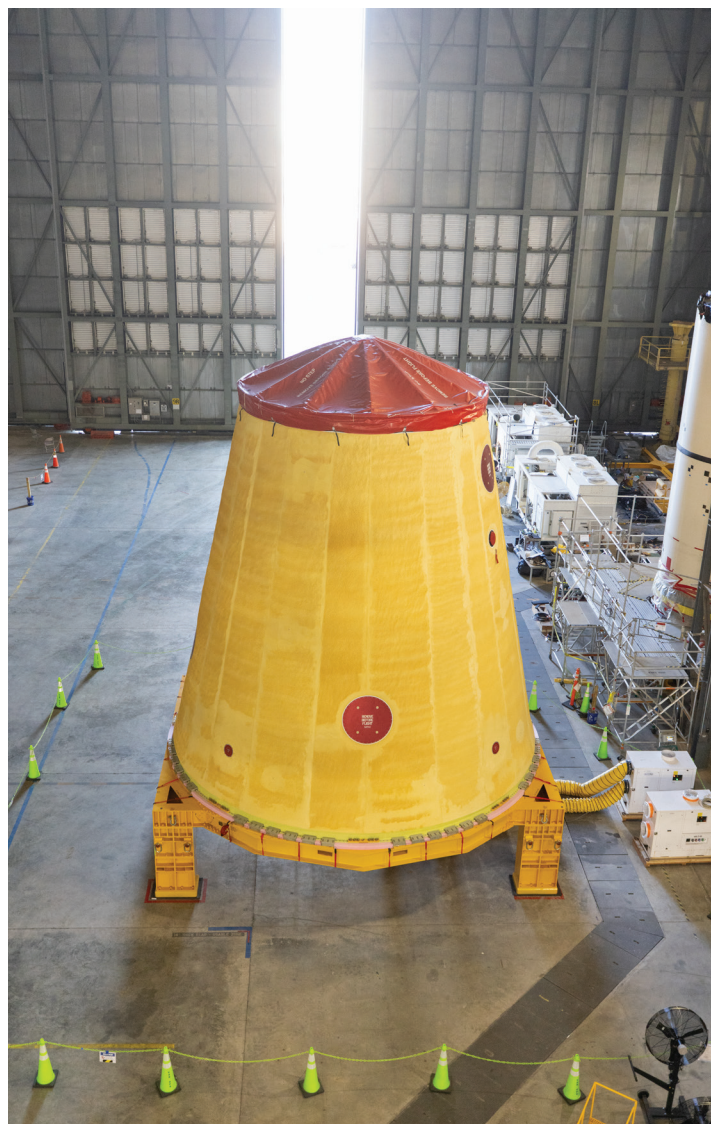
Teledyne Brown Engineering is the lead contractor for the launch vehicle stage adapter that has a pneumatically activated frangible joint that separates it and the core stage from the ICPS, Orion stage adapter, and Orion spacecraft during flight.
