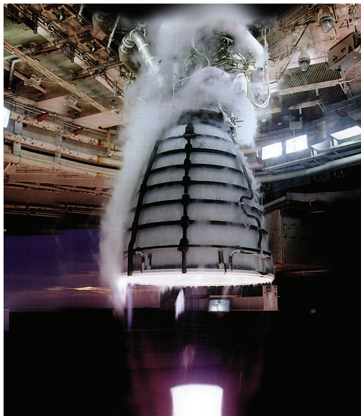
The RS-25s have been upgraded with new controllers that were hot fire tested prior to the Artemis I flight.
