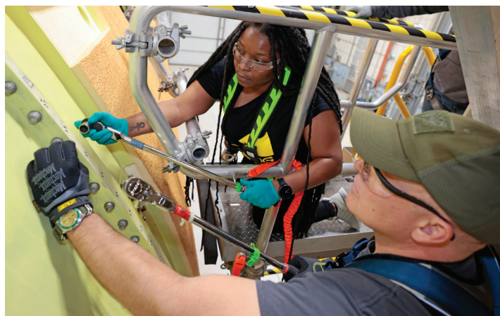
Engineers at NASA Michoud inserted 360 bolts to connect the forward assembly to the liquid hydrogen tank to make up the bulk of the core stage.
