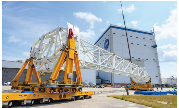
The Dynamic Demonstration Unit allows workers to practice handling the SLS core stage.
