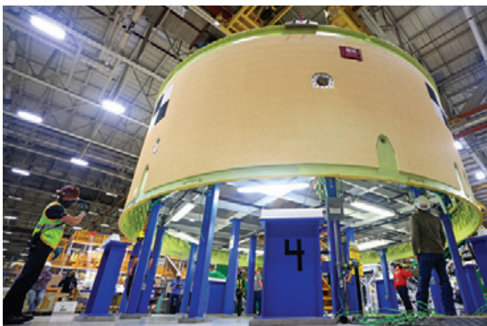
The Artemis II core stage forward skirt is seen here undergoing outfitting at NASA Michoud.
