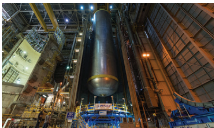
The Artemis II core stage liquid hydrogen tank is seen here readied for the next production phase at NASA Michoud.
