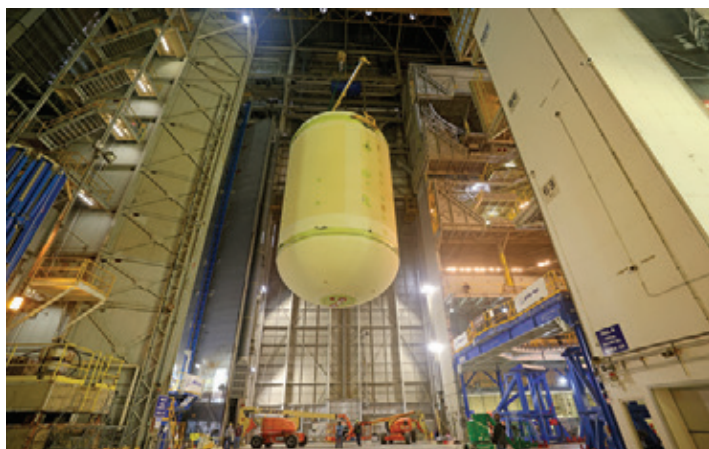
Manufactured at NASA Michoud, the Artemis II liquid oxygen tank seen here will hold up to 196,000 gallons of liquid oxygen cooled to -297 degrees Fahrenheit.
