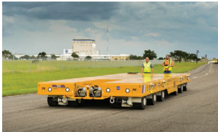
Engineers test drove a self propelled modular transporter used to carry the SLS core stage at NASA Michoud.
