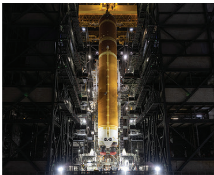
The SLS core stage, the tallest rocket stage NASA has ever built, is seen here being lowered between the Artemis II boosters in the Vehicle Assembly Building.
