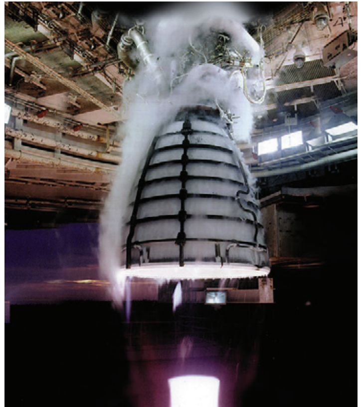
The RS-25s have been upgraded with new controllers that were hot fire tested prior to the Artemis I flight.
