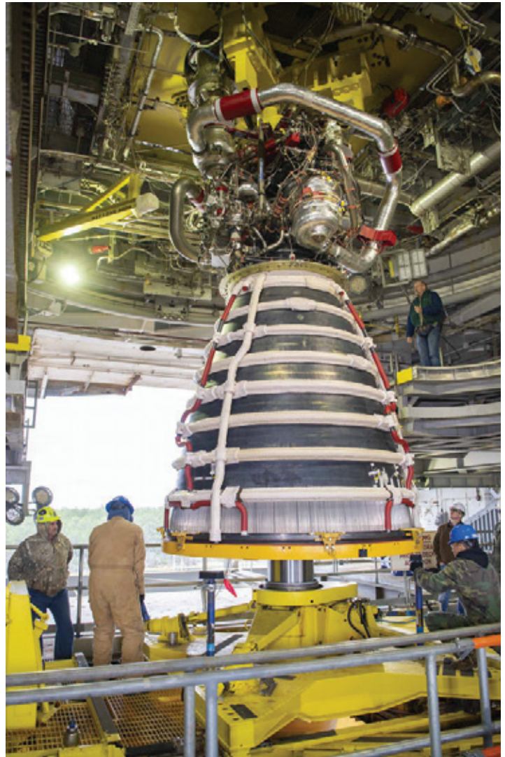
Technicians at NASA Stennis are seen preparing an RS-25 engine at the Fred Haise Test Stand.
