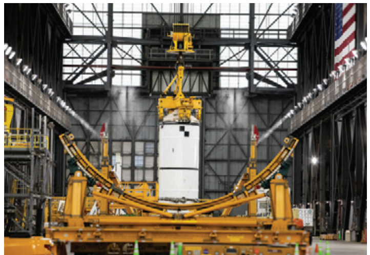
An Artemis II booster segment is seen here being lifted from its ground support equipment transportation cradle and readied for lifting with its “four point lifting beam” in the VAB.
