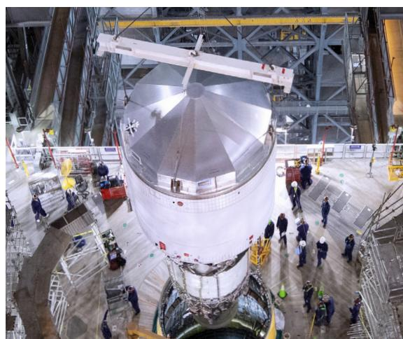
*The Artemis II SLS ICPS mates with the launch vehicle stage adapter atop the SLS core stage in the vehicle assembly building at NASA's Kennedy Space Center in Florida. The ICPS will fire its RL10 engine twice to help send the Orion spacecraft to the Moon.*
