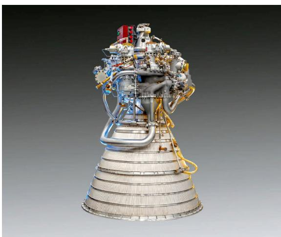
*A single RL10 engine will provide nearly 25,000 pounds of thrust and serve as the main propulsion for the interim cryogenic propulsion stage (ICPS) that is flying atop the SLS (Space Launch System) Block 1 rocket in support of each of the first three Artemis missions.*
