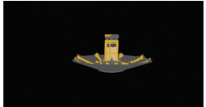
This illustration shows how the technology opens like an umbrella to slow descent and protect the payload. Credits: NASA
