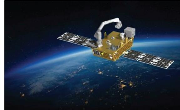
*Artist concept of the FFR Mission's robotic system payload atop the Astro Digital spacecraft. The robotic arm, provided by Motiv Space Systems, will perform robotic demonstrations in orbit. Credit: Motiv Space Systems*
