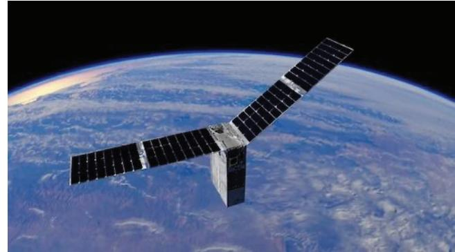
*NASA's Starling six-month mission will use a team of four CubeSats in low-Earth orbit to test technologies that let spacecraft operate in a synchronized manner without resources from the ground. Credit: NASA/Ross Walter*
