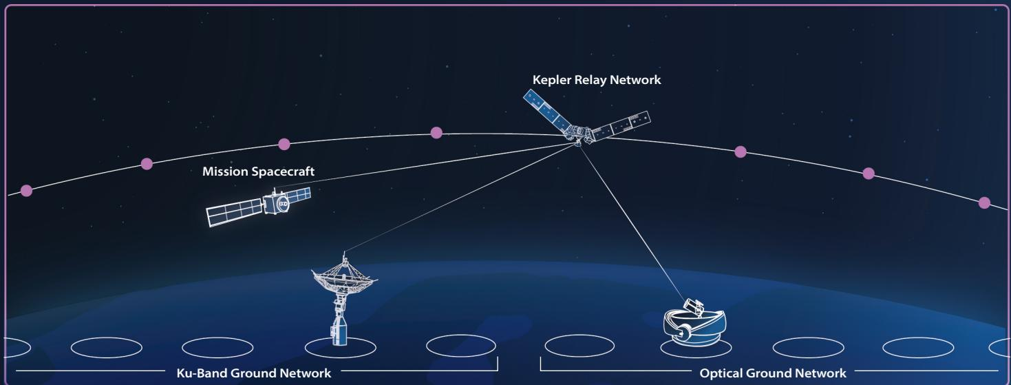
Kepler plans to deliver data through an SDA-compatible optical data relay network, connecting space and Earth communications with low latency, high throughput, and enhanced security. The Kepler Network plans to provide complete coverage of LEO above 400 km altitude.
