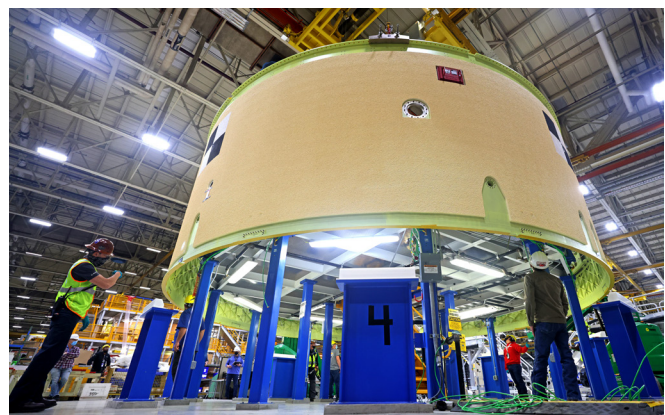
The Artemis II core stage forward skirt undergoes outfitting at Michoud. (NASA) ▲
