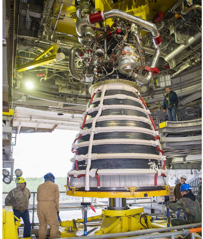
Technicians at Stennis prepare an RS-25 engine at the Fred Haise Test Stand. (NASA) ▲
