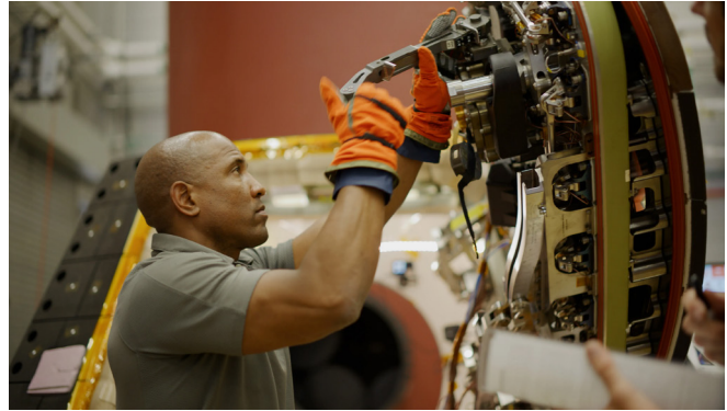
Astronaut and Artemis II Pilot Victor Glover maneuvers the latch handle on an Orion test side hatch during performance evaluations at the Lockheed Martin Space campus in Littleton, Colorado. (Lockheed Martin) ▲
