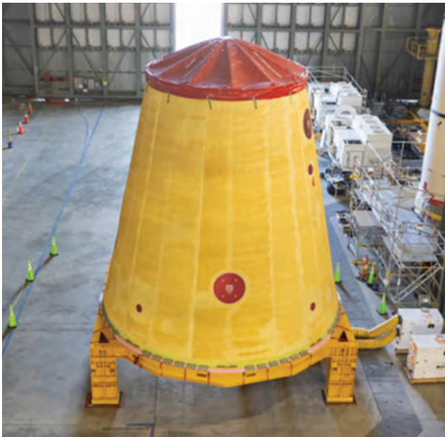
Teledyne Brown Engineering is the lead contractor for the launch vehicle stage adapter, which has a pneumatically activated frangible joint that separates it and the core stage from the ICPS, Orion stage adapter, and Orion spacecraft during flight. (NASA) ▲
