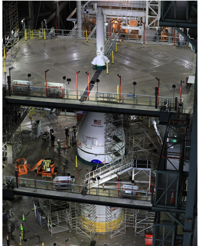
NASA's Artemis II Orion spacecraft, with its launch abort system, is stacked on the agency's SLS (Space Launch System) rocket in High Bay 3 of the vehicle Assembly Building at NASA's Kennedy Space Center in Florida on Oct. 20, 2025. (NASA/Kim Shiflett) ▲
