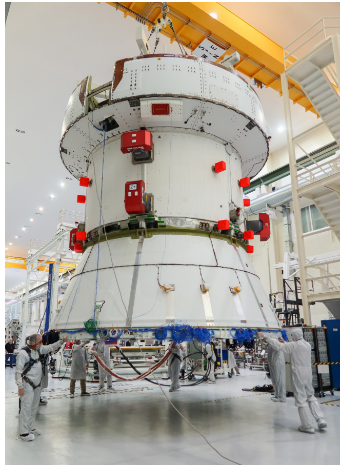
The European Service Module for NASA's Artemis II mission is lifted by crane and moved along the center aisle of the high bay inside the Neil A. Armstrong Operations and Checkout Building at NASA's Kennedy Space Center in Florida on May 22, 2023. (NASA/Amanda Stevenson) ▲
