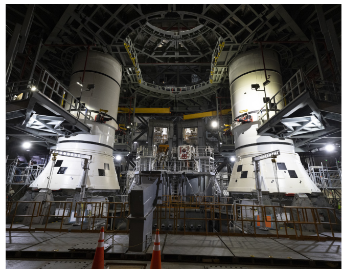
Artemis II booster aft assemblies are pictured here on the mobile launcher in the Vehicle Assembly Building. (NASA) ▲
