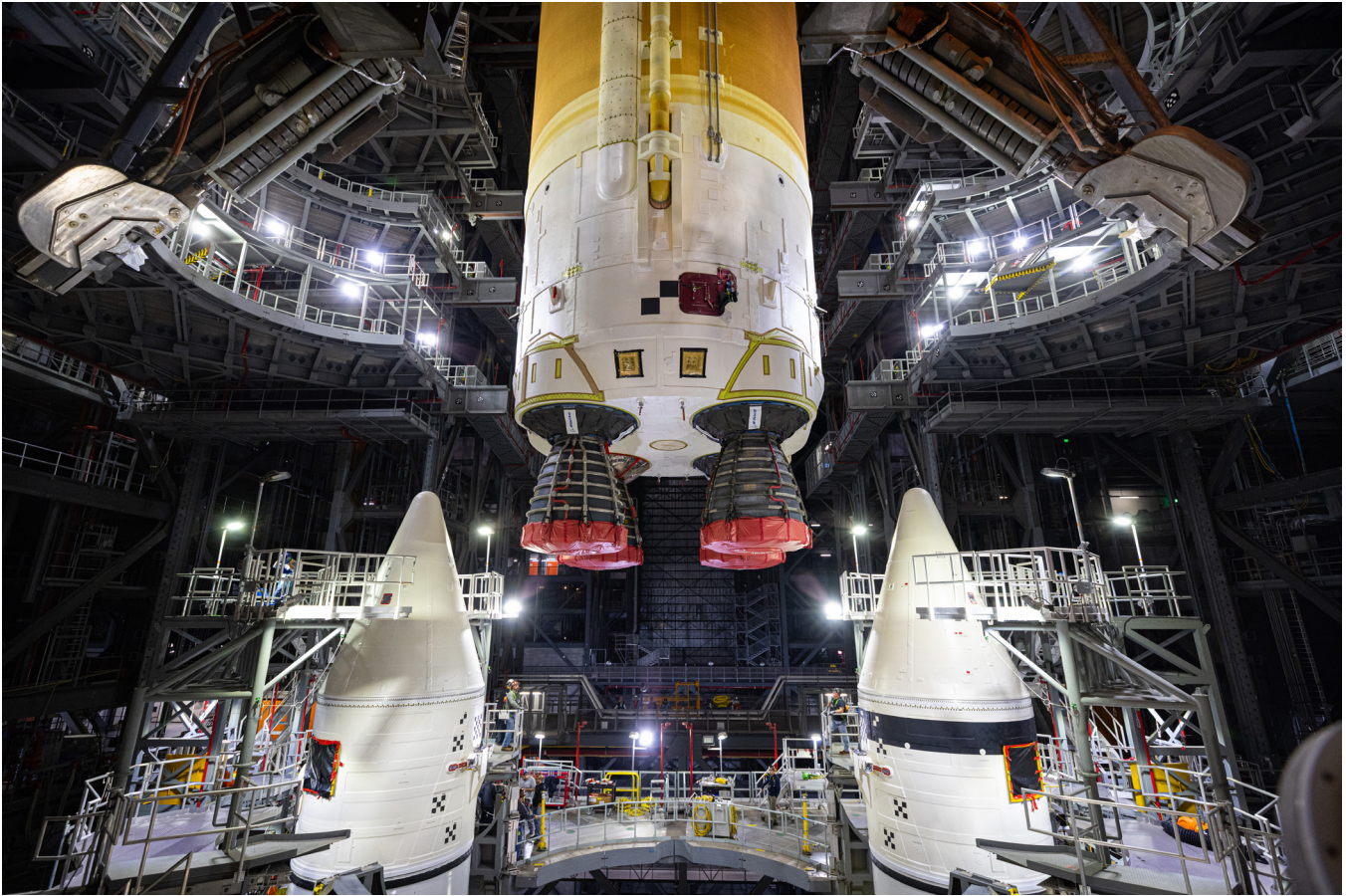
The Artemis II core stage is seen here being lowered between the SLS solid rocket boosters in the Vehicle Assembly Building at NASA's Kennedy Space Center. (NASA) ▲
