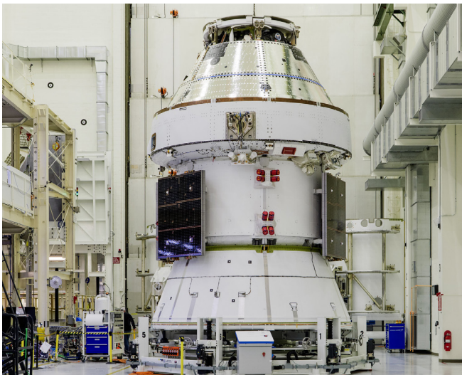
The four solar array wings for the Artemis II Orion spacecraft are installed inside the Operations and Checkout Building at NASA's Kennedy Space Center in Florida on March 7, 2025. (NASA) ▲
