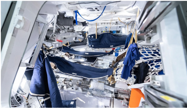
Artemis II crew sleeping bag configurations are tested in the Orion spacecraft medium-fidelity mock-up at NASA's Johnson Space Center in Houston, as well as used for astronaut training and systems familiarization. (NASA) ▲
