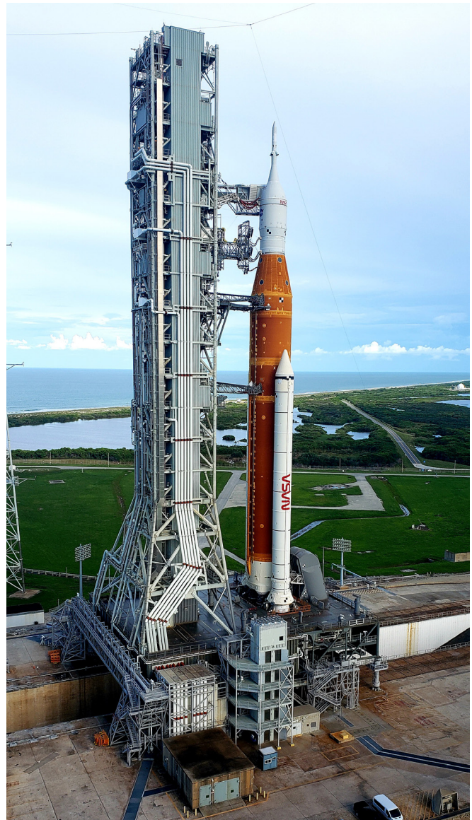
A close-up view of the Artemis I SLS (Space Launch System) rocket and Orion spacecraft atop the mobile launcher on Launch Pad 39B. (NASA) ▲
