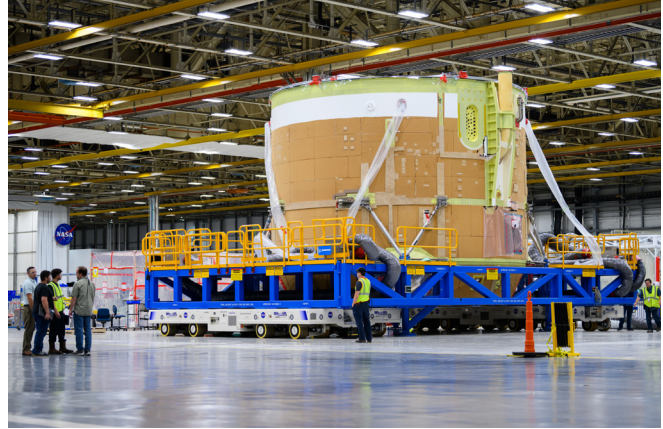
Workers at Michoud are seen here moving the Artemis II core stage engine section. (NASA) ▲
