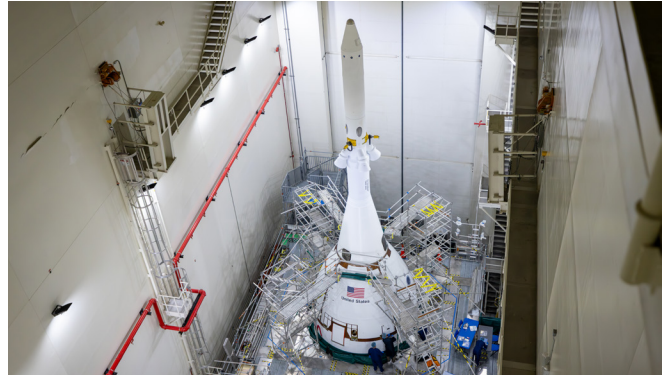
Teams with NASA's Exploration Ground Systems attached the fourth and final ogive fairing for the launch abort system of the Orion spacecraft for the Artemis II mission. The fully installed fairings were photographed inside the Launch Abort System Facility high bay at NASA's Kennedy Space Center in Florida on Sept. 17, 2025. (NASA/Frank Michaux) ▲
