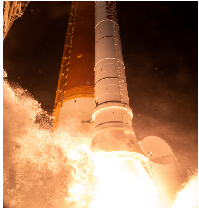
A bird’s eye view of the Artemis I launch shows one of the rocket’s solid rocket boosters shortly after ignition. (NASA/Chris Coleman, Kevin Davis) ▼
