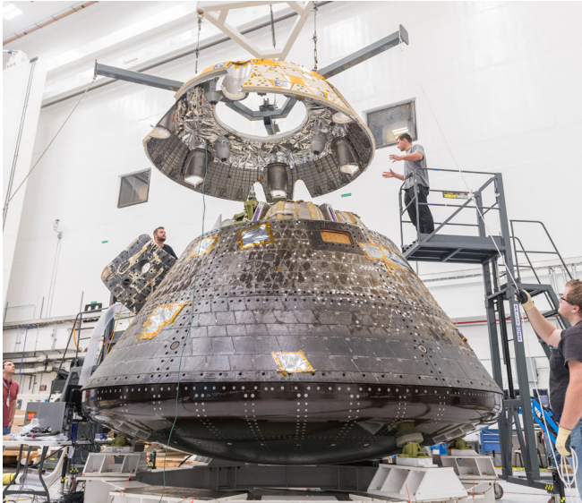
The Artemis I Orion crew module, also known as the Orion Environmental Test Article, prepares for testing with installation of the forward bay cover. The crew module returned to NASA's Neil Armstrong Test Facility in Sandusky, Ohio, in January 2024 and completed an 11-month test campaign necessary for the safety and success of Artemis II. (NASA/Jordan Salkin) ▲
