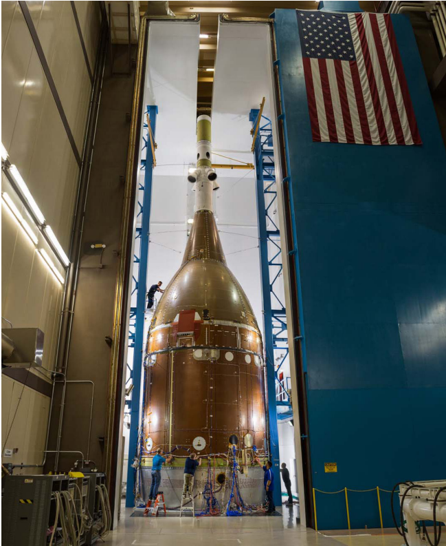
NASA's Orion structural test article in its "full stack" launch configuration at Lockheed Martin Space in 2018. (Lockheed Martin) ▲
