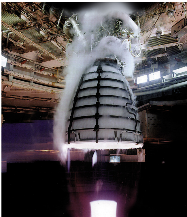
The RS-25 engines were upgraded with new controllers that were hot-fire tested prior to the Artemis I test flight. (NASA) ▲
