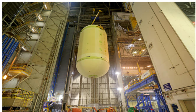
Manufactured at Michoud, the Artemis II liquid oxygen tank, seen here, holds up to 196,000 gallons of liquid oxygen cooled to -297 degrees Fahrenheit. (NASA) ▲
