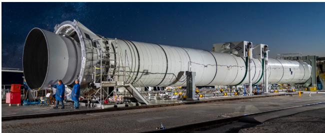
A close-up of the Flight Support Booster-2 solid rocket motor, poised for a full-scale ground test at Northrop Grumman's Utah test facility. (NASA) ▲
