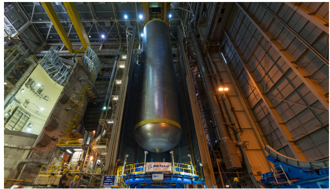
The Artemis II core stage liquid hydrogen tank is readied for its next production phase at Michoud. (NASA) ▲
