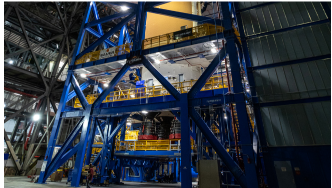
Teams with EGS lower the 212-foot-tall SLS core stage into High Bay 2. (NASA) ▲
