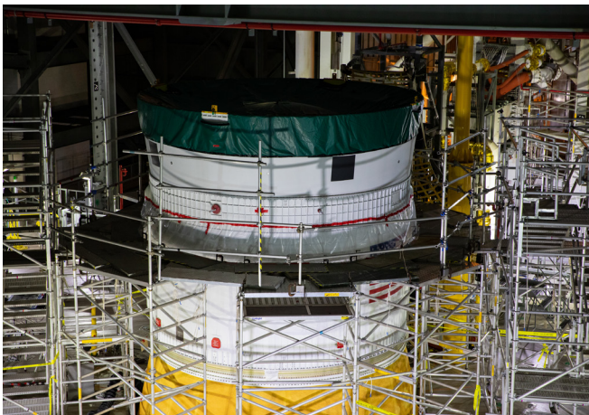
The Orion stage adapter is the final element of SLS to be stacked before the Orion spacecraft is added. The Artemis I Orion stage adapter was covered to protect the mission's secondary payloads prior to the addition of the spacecraft. (NASA) ▲
