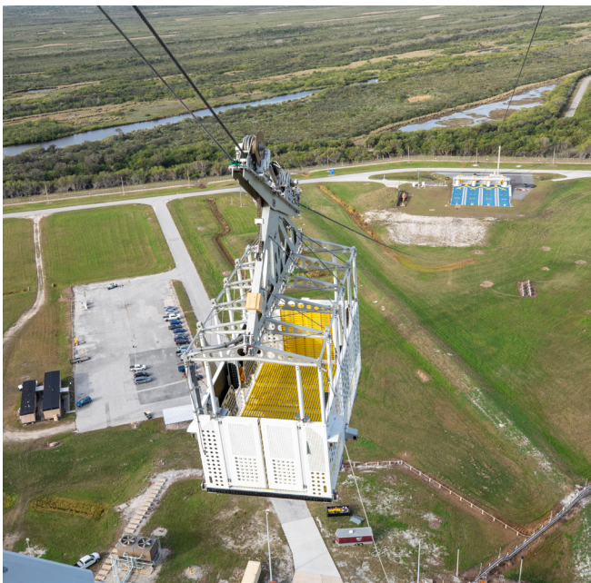
One of the four emergency egress baskets on the mobile launcher as it is lowered to the terminus site. (NASA/Isaac Watson) ▲
