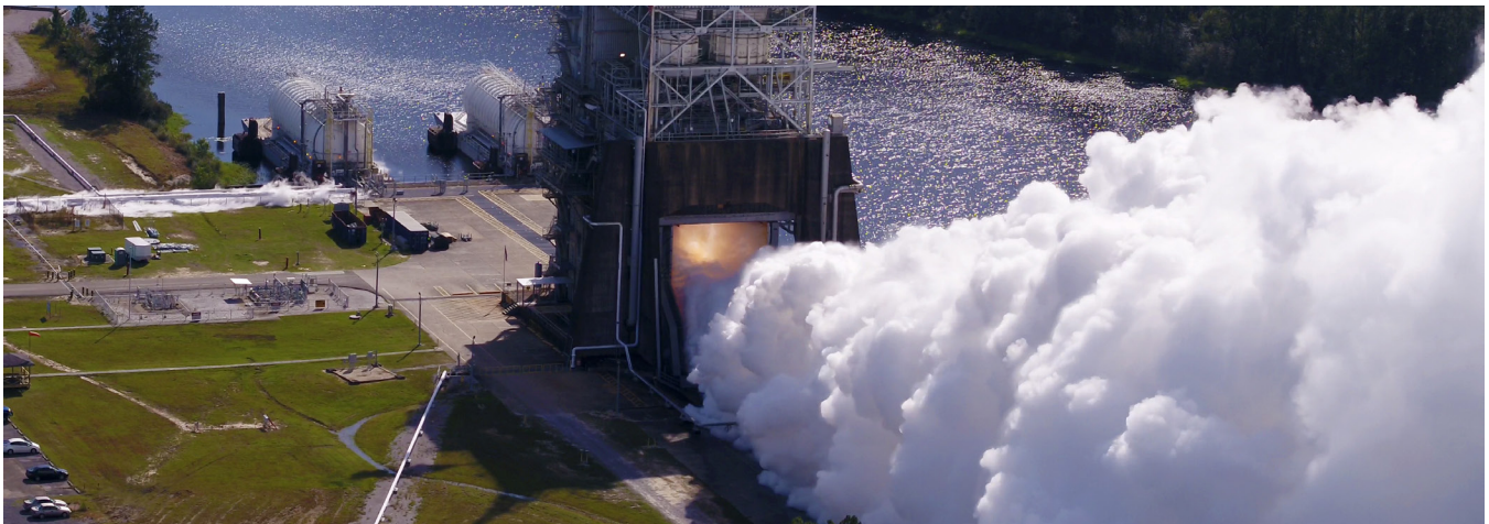
Dedicated ground test RS-25 engines were fired at Stennis to qualify engines to specific SLS operating conditions. (NASA) ▲
