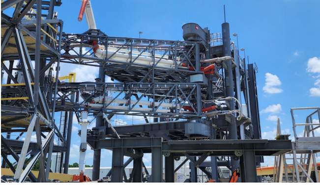
Umbilicals being tested at the Launch Equipment Test Facility. (NASA) ▲
