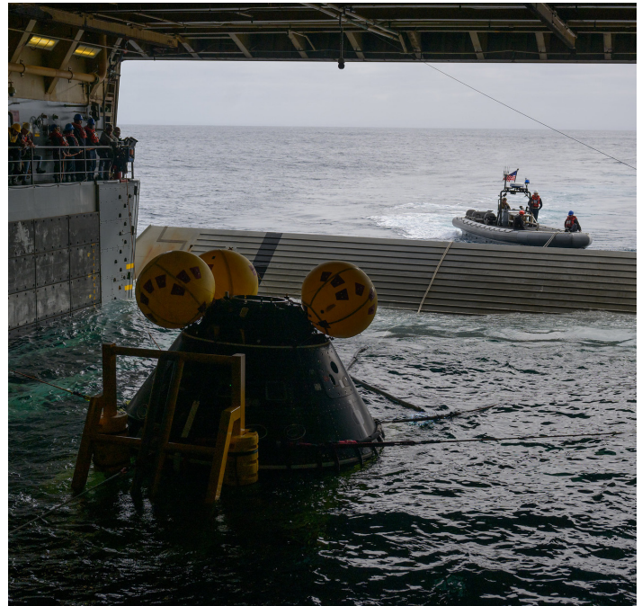
Teams recover the Crew Module Test Article — a full-scale mock-up of the Orion spacecraft — as they practice Artemis recovery operations during Underway Recovery Test-12 aboard USS Somerset off the coast of California on March 29, 2025. During the test, NASA and Department of War teams practice recovery procedures for NASA's Artemis II mission around the Moon, which will conclude with splashdown in the Pacific Ocean. (NASA/Bill Ingalls) ▲
