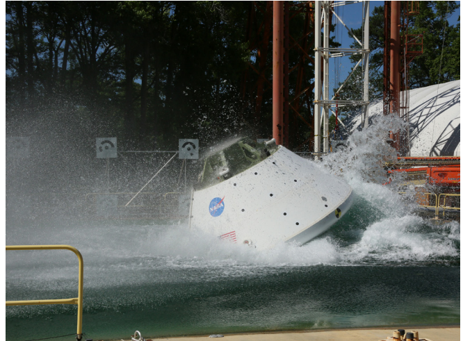
The Orion Ground Test Article completes its first swing water impact test at NASA's Langley Research Center in Virginia on June 8, 2016. (NASA/David C. Bowman) ▲
