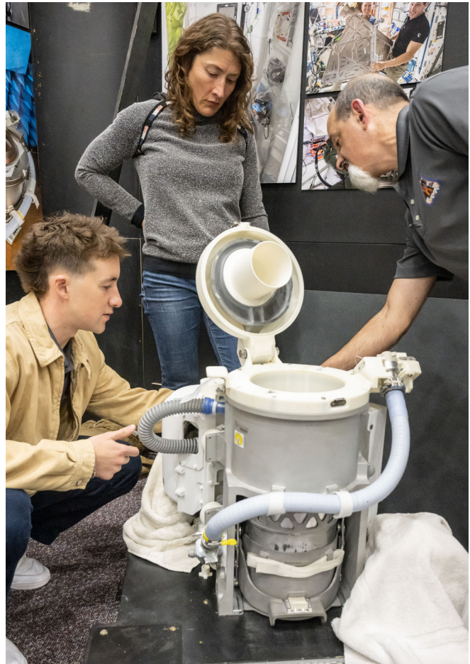
Artemis II astronaut Christina Koch receives training on the Orion Universal Waste Management System at NASA's Johnson Space Center. (NASA) ▲
