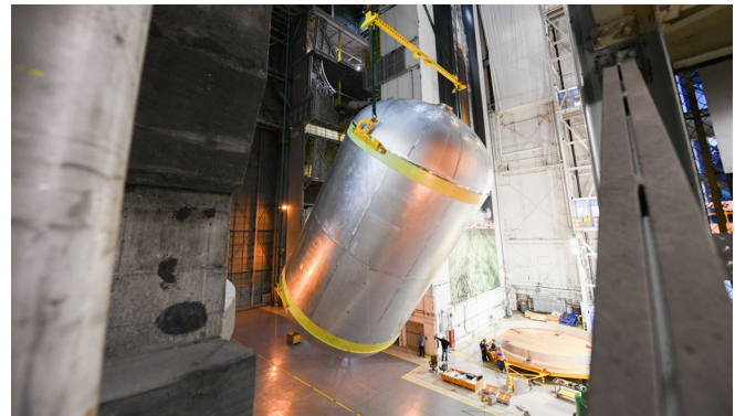
The Artemis II core stage liquid oxygen tank is seen here after cleaning as it is prepared to move to another area for spray insulation at Michoud. (NASA) ▲
