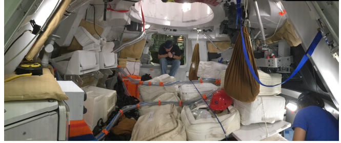
Engineers conduct testing in a representative Orion vehicle at NASA's Johnson Space Center to evaluate procedures that will be used to protect astronauts during radiation events in space. (NASA) ▲
