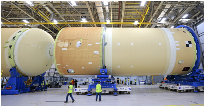
Workers at NASA's Michoud Assembly Facility in New Orleans prepare to join the core stage liquid hydrogen tank (left) to the core stage forward assembly, comprising the forward skirt, liquid oxygen tank, and intertank. (NASA) ▲
