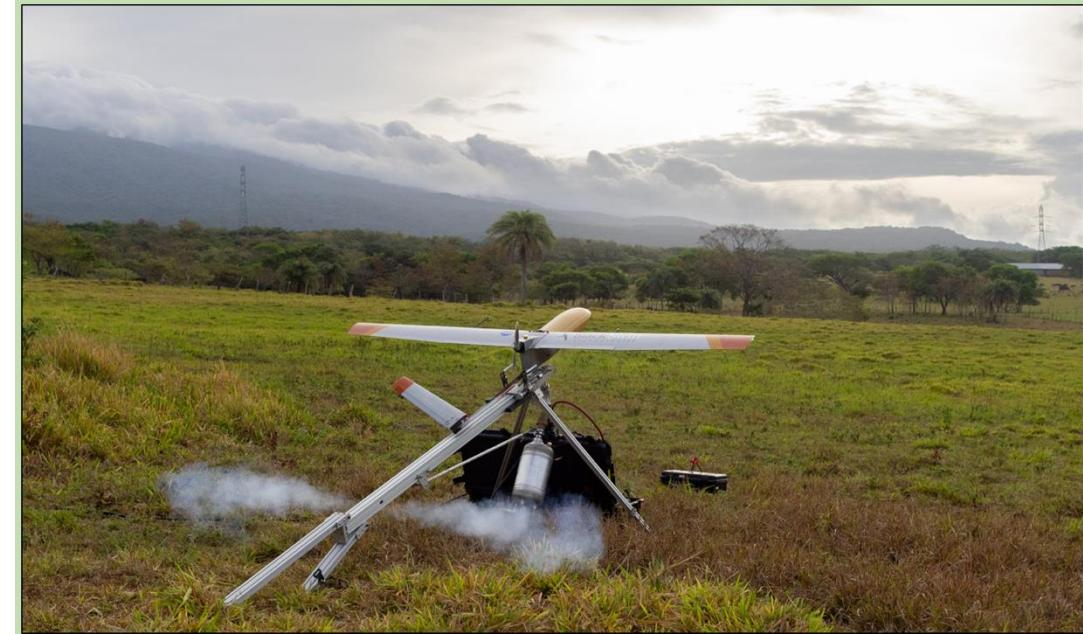
**NASA ARC Black SwiftTM S2 UAS take-off.** The catapult-launched, electric-powered fixed-wing S2 UAS carries a 5-pound science payload for over 60 minutes and can reach targets more than 20 miles away. Its capability for stand-off launches and recovery enables operations in complex, remote terrain without requiring an airfield. The modular platform with field-swappable payload cones supports sorties in agile succession.
