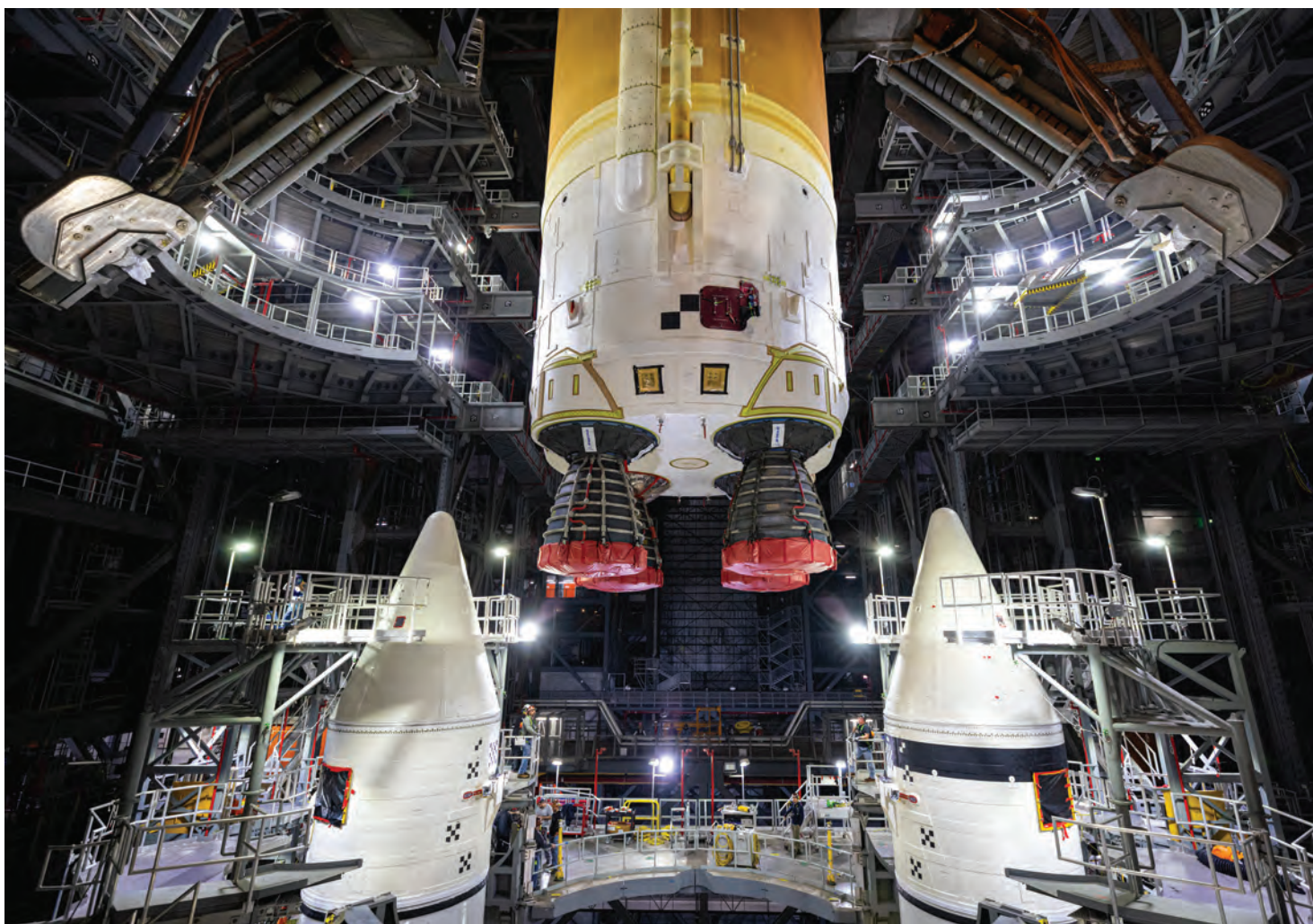
The Artemis II core stage is seen here being lowered between the SLS solid rocket boosters in the Vehicle Assembly Building. The SLS design uses a proven propulsion system of solid rocket boosters and liquid-fueled RS-25 engines to launch more payload to the Moon than any rocket since the Saturn V.
