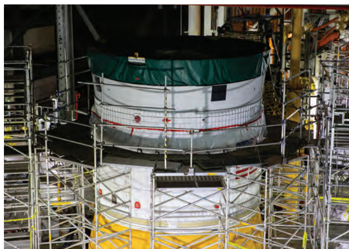
The OSA is the final element of SLS to be stacked before the Orion spacecraft is added. The Artemis I OSA was covered to protect the mission's secondary payloads prior to the addition of the Orion spacecraft.
