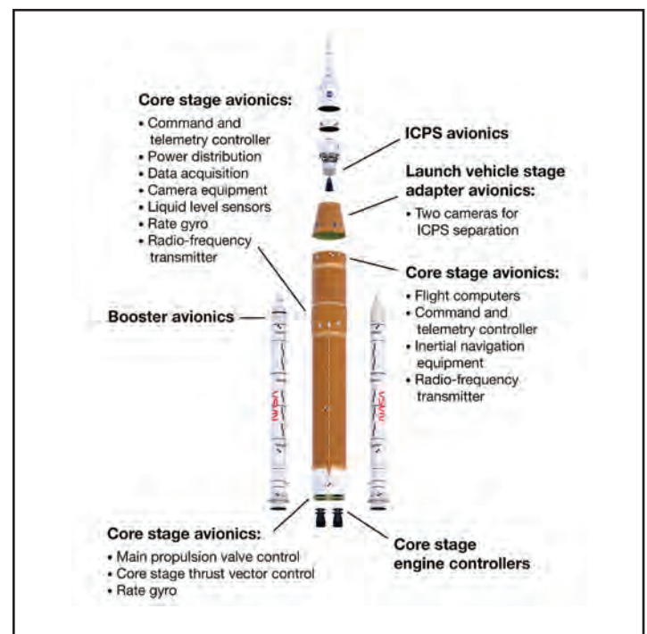
Avionics throughout the elements of SLS monitor the rocket's health and control the flight.
