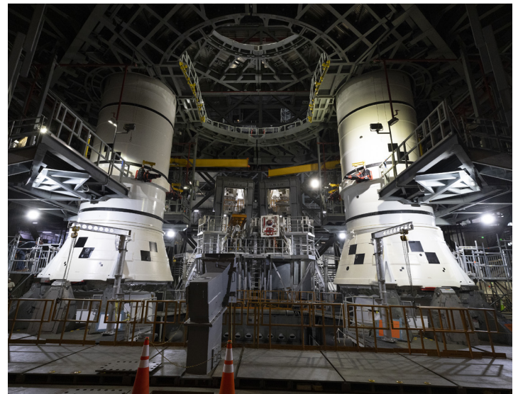
Artemis II booster aft assemblies are seen here on the mobile launcher in NASA Kennedy's Vehicle Assembly Building.
