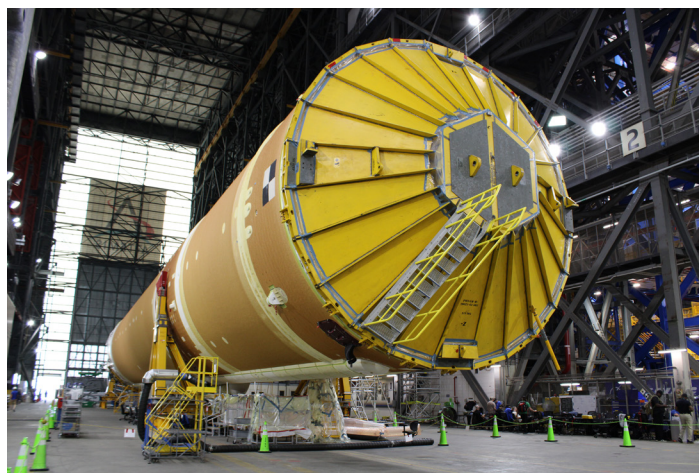
A lifting fixture called a "spider" is seen here attached to the Artemis II core stage in the VAB.
