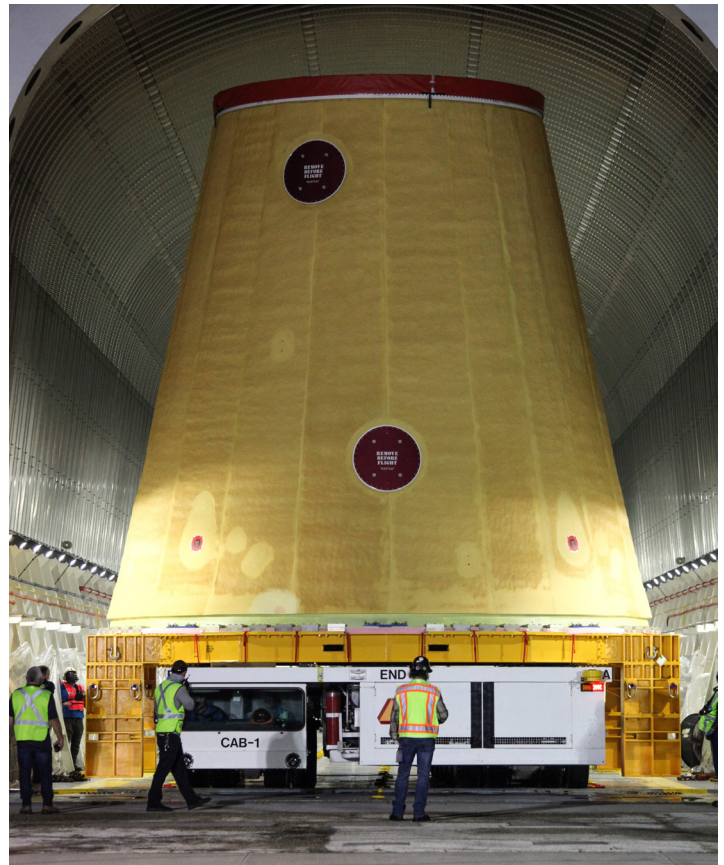
The LVSA partially encloses the ICPS and contains the pyrotechnic system to separate itself and the core stage from the ICPS and Orion spacecraft.
