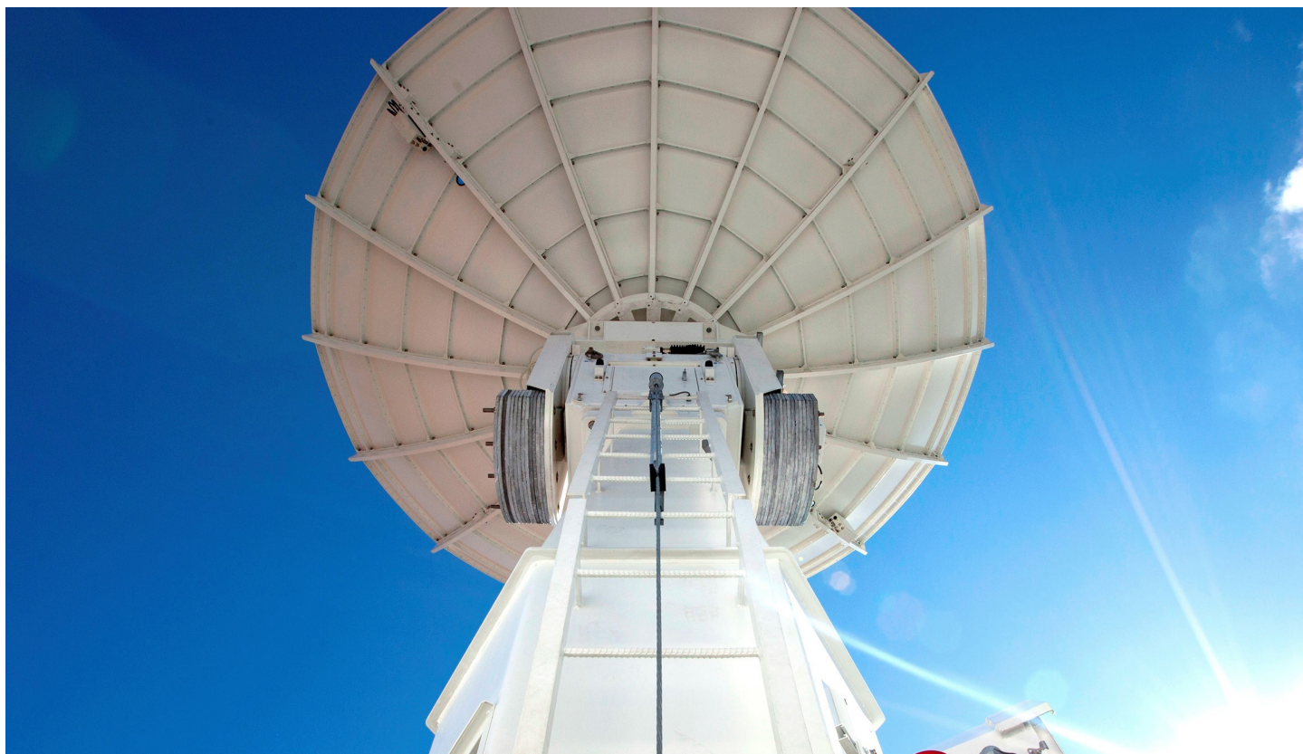
Part of the Kennedy Uplink Station, the S-band ground tracking system at NASA Kennedy provides crucial tracking and communication capabilities following liftoff of SLS and Orion.
