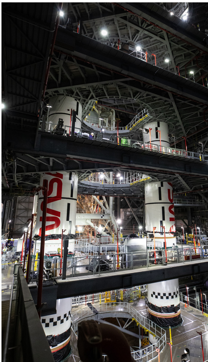
The completed Artemis II boosters are shown stacked on the mobile launcher in the Vehicle Assembly Building at NASA Kennedy before integrating the other elements of SLS and Orion.
