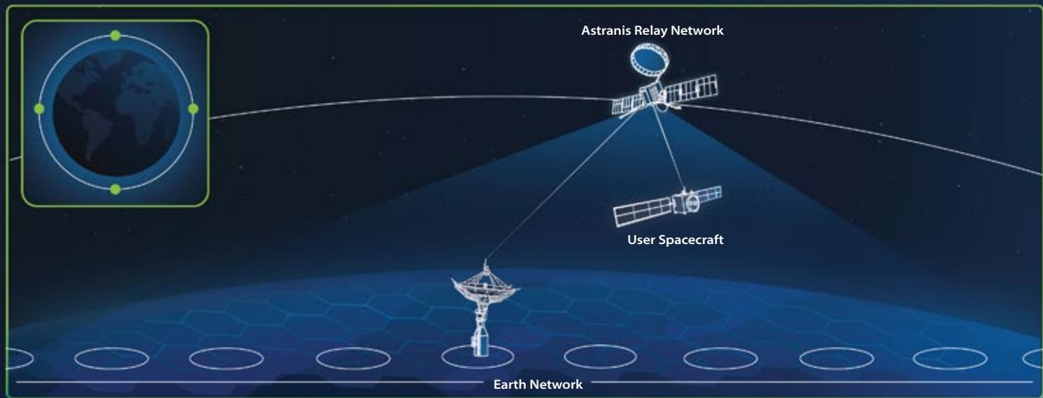
Satellite relay services will be enabled by clusters of Astranis Omega spacecraft, spaced approximately 90 degrees apart in geostationary orbit, providing completed global coverage.
