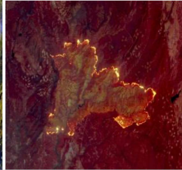
MASTER images of the Mosquito fire. Left image: 2.1 \mu\text{m} , 1.6 \mu\text{m} , 0.54 \mu\text{m} bands; Right image: 4 \mu\text{m} , 2.1 \mu\text{m} , 1.6 \mu\text{m} bands. Note the exclusion of smoke in the right image by only using the thermal bands.
