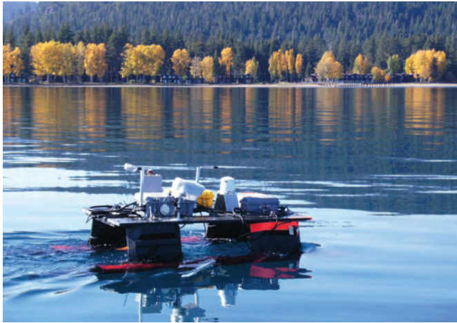
SWATH Boat During a Bathymetric Mapping Mission in Lake Tahoe
