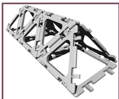
Truss design using Transformable Robotic Infrastructure-Generating Object Network (TRIGON)
