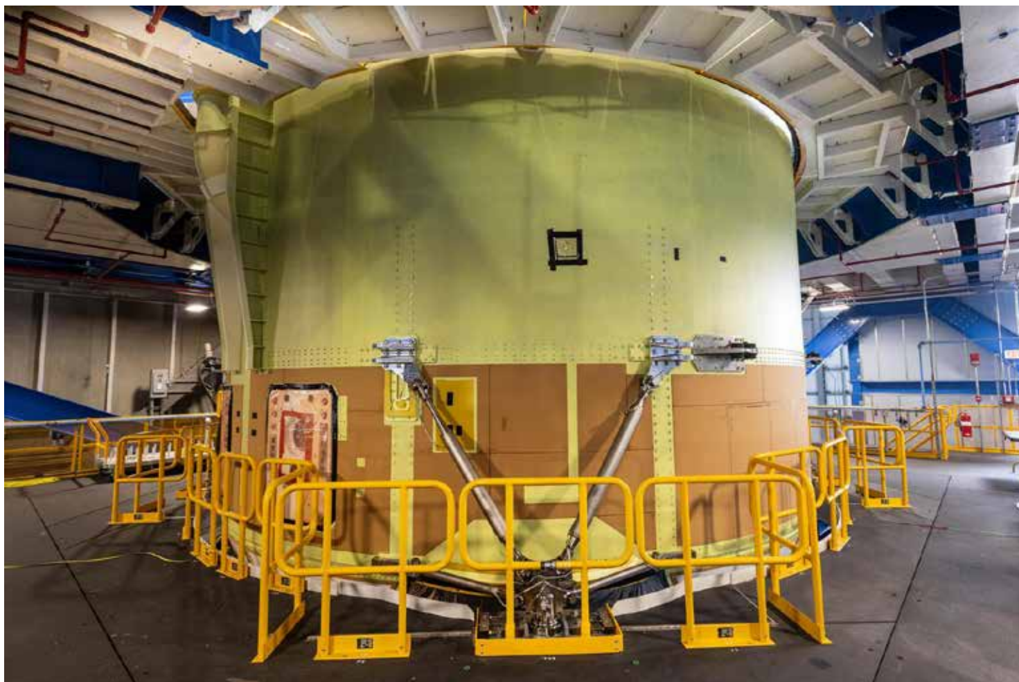
Teams from NASA Kennedy prepare to lift NASA's integrated Artemis III SLS core stage engine section with its boat-tail inside the center's Vehicle Assembly Building in August.
