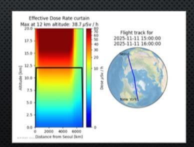
NAIRAS model real-time predictions for a transpolar commercial aircraft during the November 2025 SEP event, taken from the CCMC. The recommended effective dose rate threshold is 20 µSv/h.
