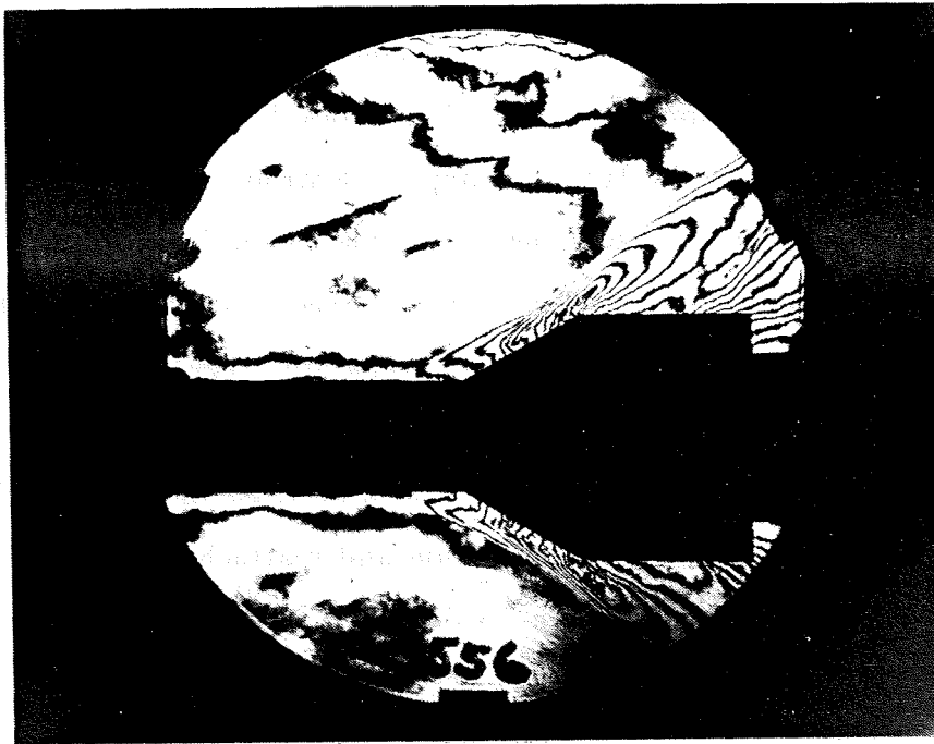
Figure 11(a). Infinite-fringe reconstruction for the 30^\circ model at M_\infty = 2.85 , P_t = 1.7 atm, and Re_L = 18 \times 10^6 .
