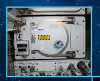
The Glacier is a double middeck locker-sized cryogenic freezer. The primary function of Glacier is to provide cryogenic preservation of science samples aboard the ISS and thermal control in visiting vehicles. Glacier is designed to support experiments that require temperatures between -95°C and +4°C for launch/return and -160°C to +4°C on ISS.
