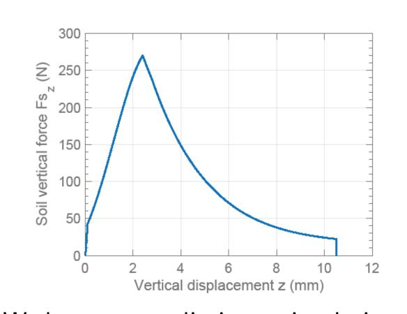
We have run preliminary simulations based on landing models of a 1 kg robot landing at 1.4 m/s (in Fillite simulant).
