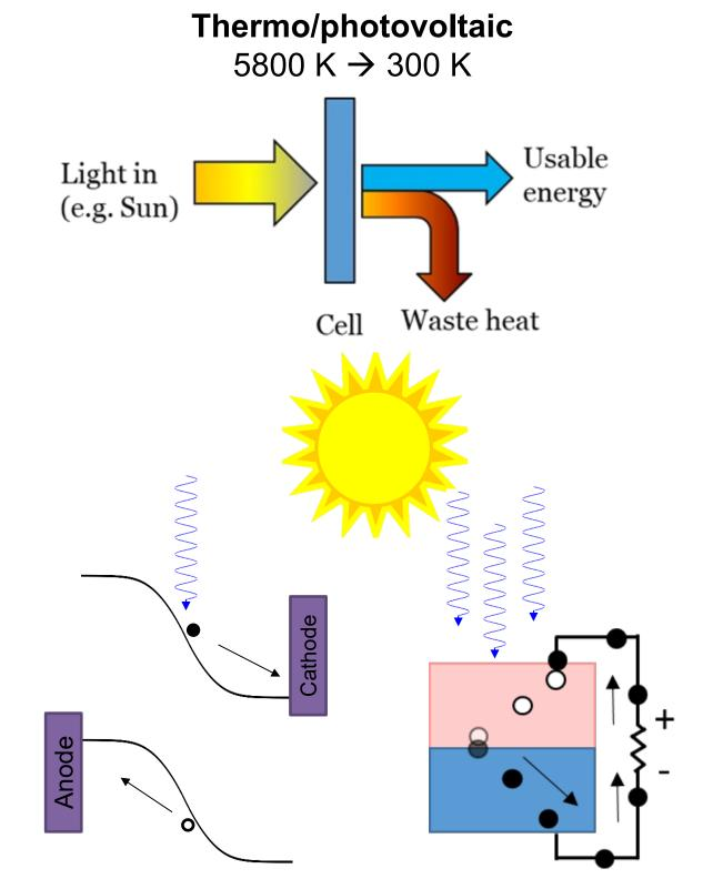
PV devices absorb photons from the hot sun, generating electron-hole pairs which are separated and collected generating a negative current at positive voltage to perform work in an external load.
