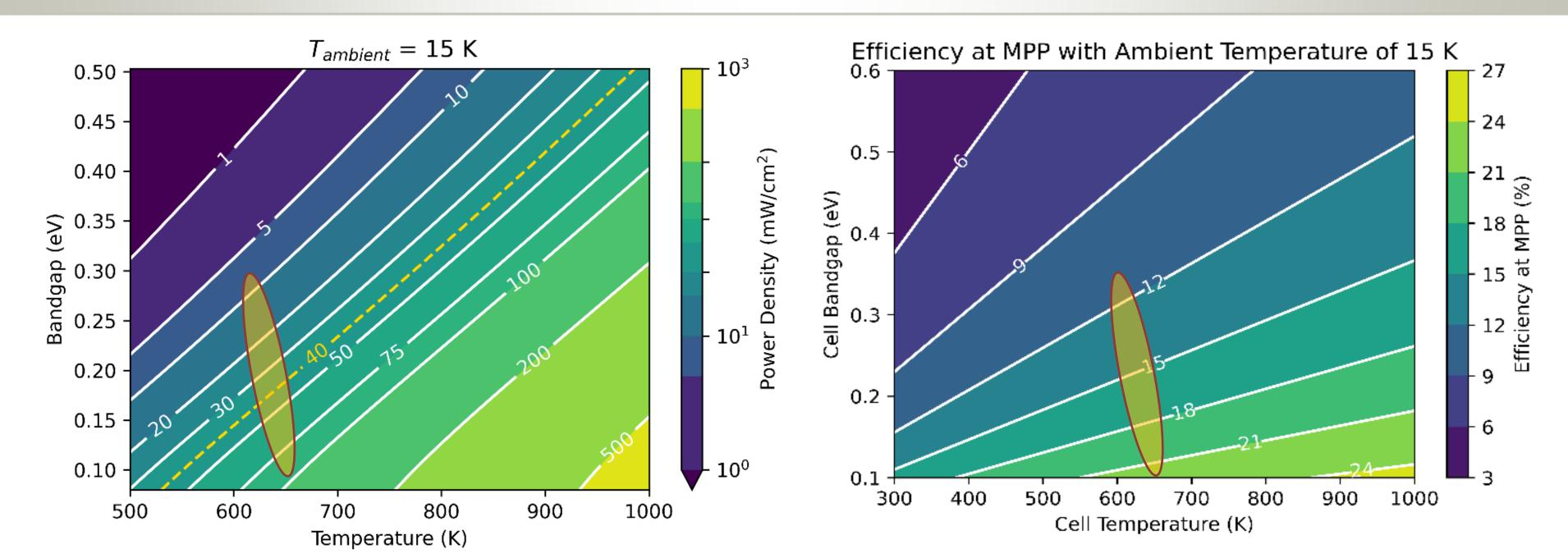
Power output levels > 6 mW/cm² at a power conversion efficiency of 12.3 % are possible in low bandgap systems
