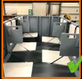
EMERGENCY EGRESS SYSTEM BASKET PROTOTYPE COMPLETE
