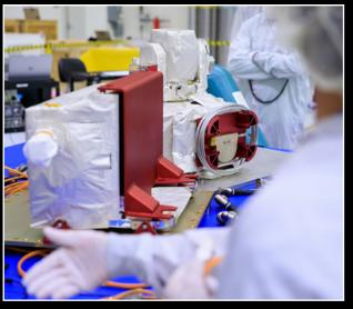
In June, the laser communications system for the Artemis II mission – O2O – arrived at Kennedy for mechanical integration with the Orion spacecraft. Mechanical integration included the installation of the inner wall assembly, optical module, and controller electronics module. Additionally, the team completed an end-to-end integrated lab test with the mission control center.
