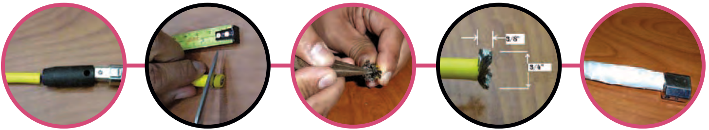
Images of the jumper cable modified to create the wire brush tool.
