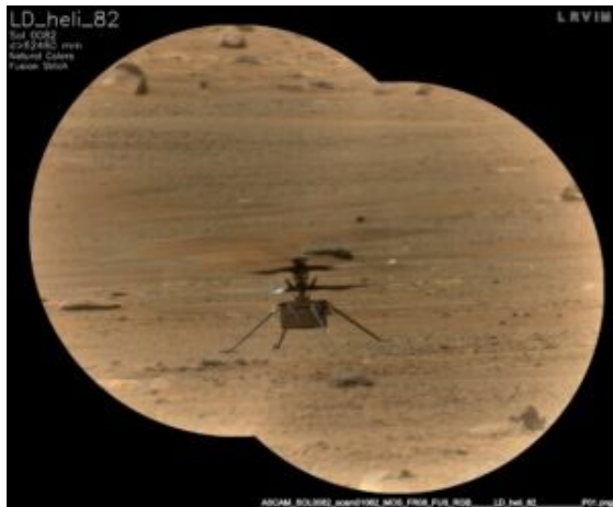
NASA’s Ingenuity Mars Helicopter is viewed here through the Remote Microscopic Imager (RMI) camera, part of the SuperCam instrument aboard NASA’s Perseverance rover. This image was taken on May 14, 2021, the 82nd Martian day, or sol, of the mission. Photo Credit: NASA/JPL
