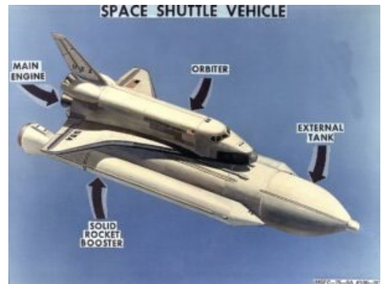
A diagram showing various parts of the space shuttle. Credit: NASA/MSFC
