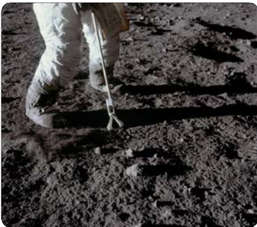
Tongs were used to pick up rock samples. Apollo 12 photograph AS12-47-6932.
