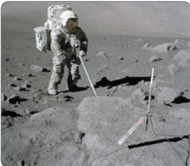
Scoops were used to collect soil samples. Several different scoop designs were used during the Apollo program. A shovel-like trenching tool was also used on one mission. Apollo 17 photograph AS17-146-22371.
