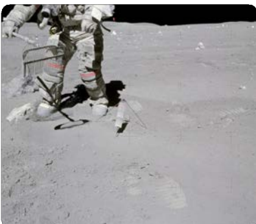
Rakes were used to collect small pebbles. The tines on the rake are 1 centimeter apart. The rake was dragged through the soil and then shaken. Small particles fell through the tines and larger particles were trapped in the rake and dumped into a sample bag for return to Earth. Apollo 16 photograph AS16-116-18629.
