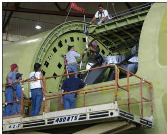
Photograph of telescope cavity installation at the L3 facility in Waco, Texas. (NASA ID: ACD03-0160-143/Eric James)
