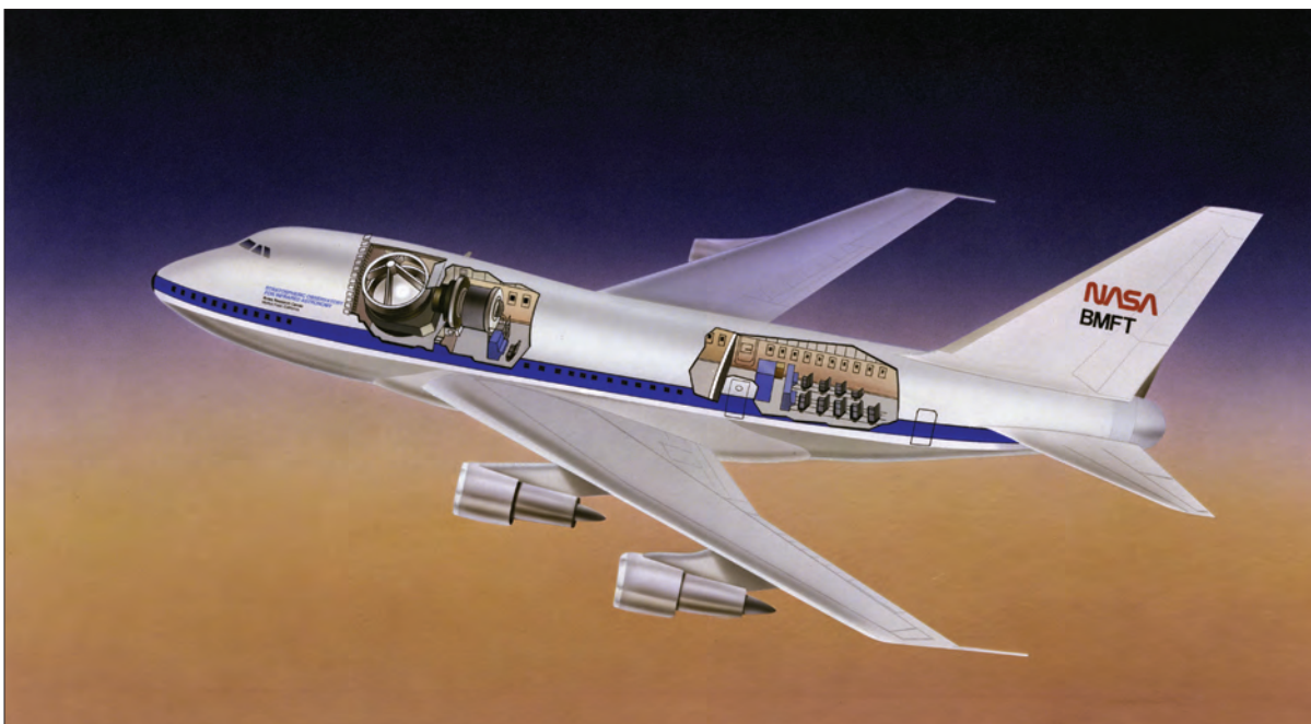
Cutaway illustration of the telescope and mission control areas from 1988. BMFT stands for the German Bundesministerium für Forschung und Technologie, or the Federal Ministry for Research and Technology. The BMFT was a central player in the development of the German space program from the 1970s through the early 1990s. (NASA ID: AC88-0371-2)
