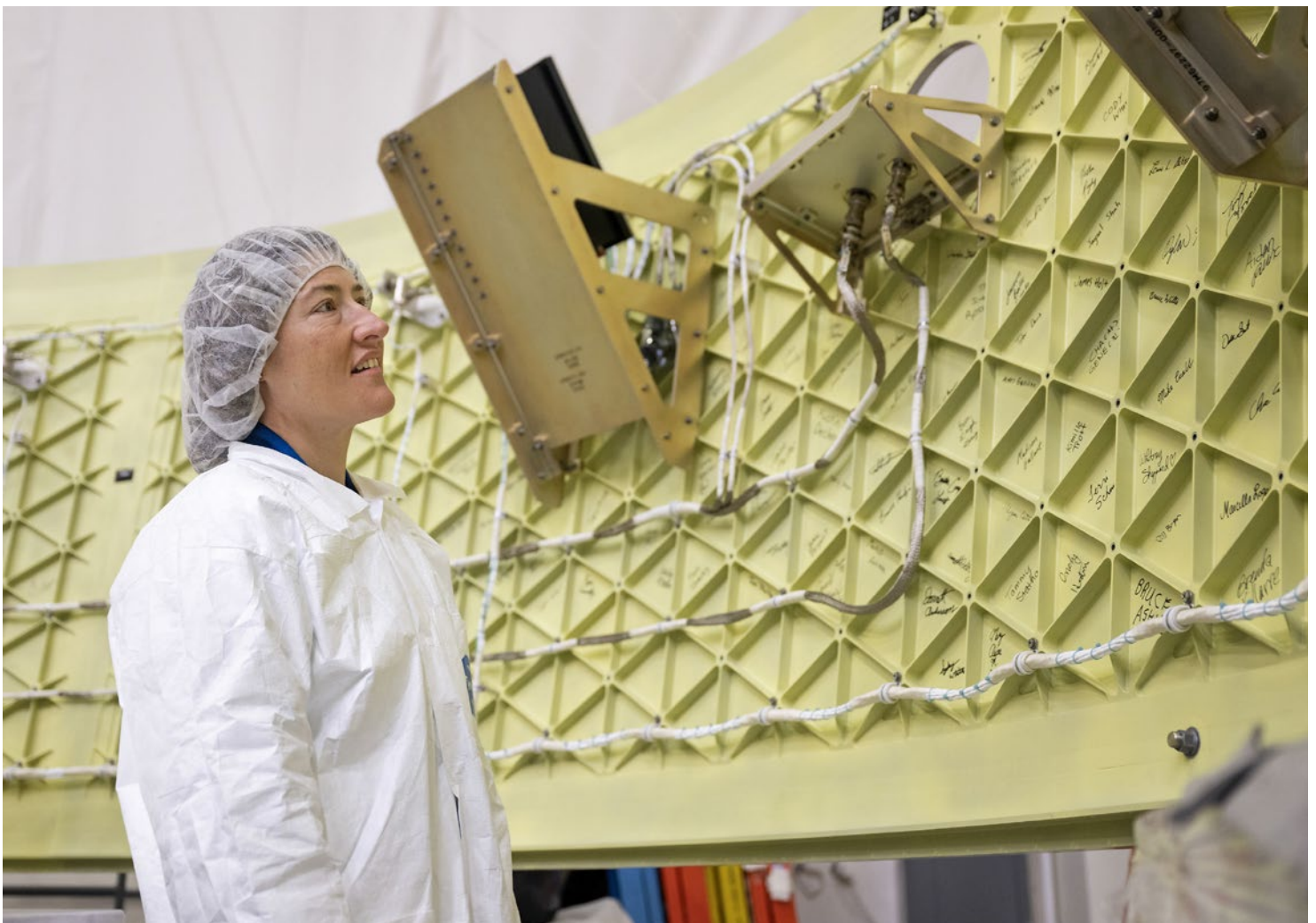
NASA astronaut and Artemis II Mission Specialist Christina Koch examines the Orion stage adapter, a ring-like structure that connects the agency's SLS rocket to the Orion spacecraft.
