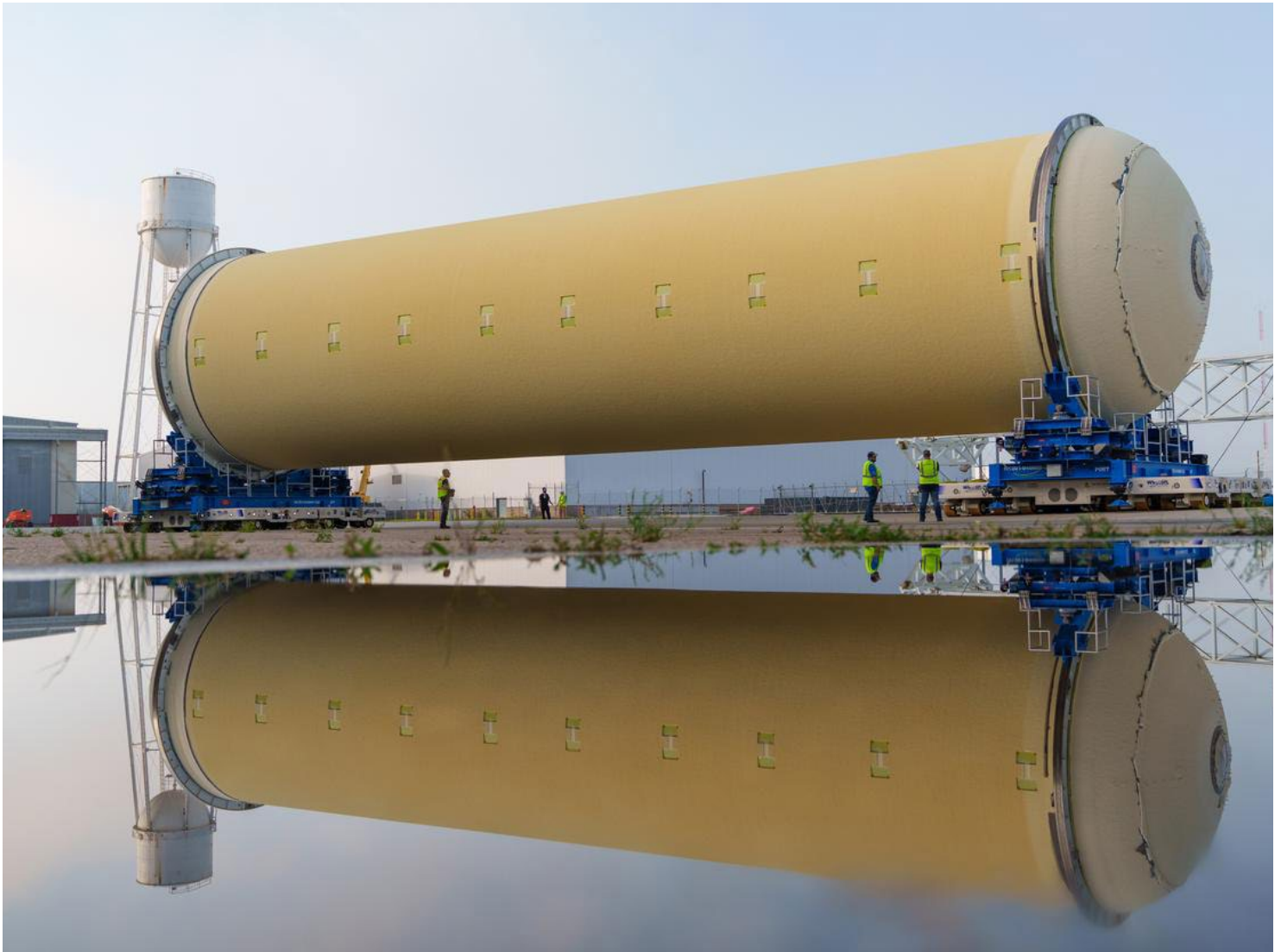
Teams at NASA's Michoud Assembly Facility in New Orleans move a liquid hydrogen tank for the Artemis III SLS into the factory's final assembly area April 22.
