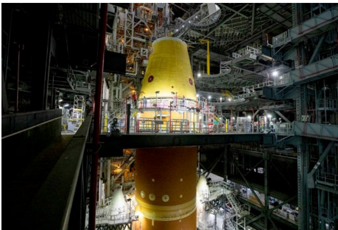
The launch vehicle stage adapter for the Artemis II SLS was added to the core stage April 12.
