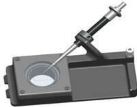
Design rendering of PACE-2 with oil dispensing syringe installed in LMM.
