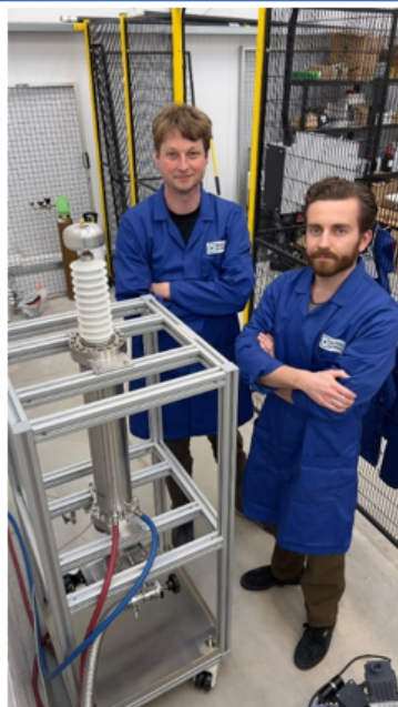
Figure 3: Tom Haywood (left) and Dr. Tom Wallace-Smith (right) from Astral Systems Ltd, together with their Gen2 research reactor. This reactor has the same internal geometry as their commercial systems but is easy to open and close at the bottom so that they can swap their many deuterium-loaded plasma-facing sleeves as they complete their own LCF experiments, searching for the best materials and manufacturing processes to maximize performance.
