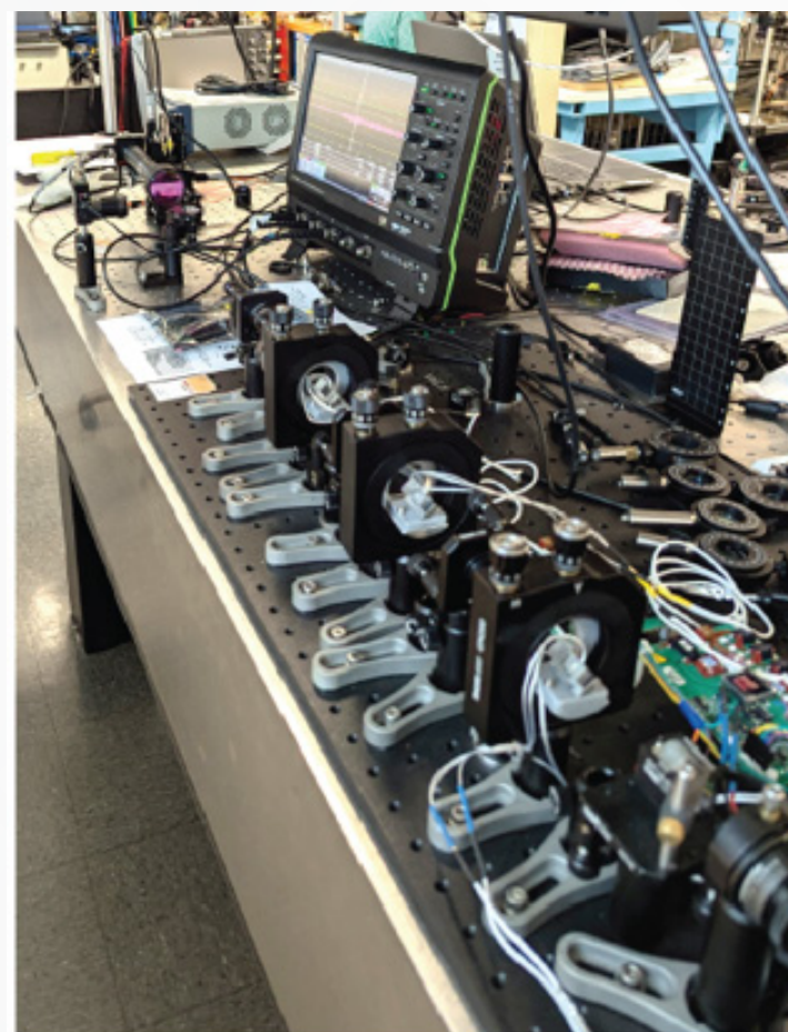
Laboratory prototype of digital beam scanner in its 8-beam configuration (L: setup, R: far-field test images of the 8 beam paths). This IRAD-funded prototype demonstrated the required crosstalk isolation, throughput efficiency, and pointing accuracy needed for space-based geodetic laser altimetry.
