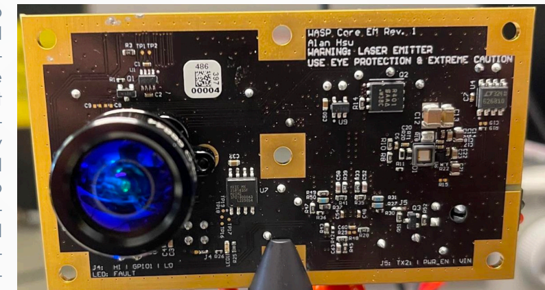
A Wearable Active Sensing Processor (WASP), which will likely be flown on an industry lunar rover in 2026.
