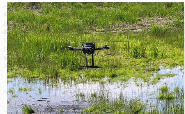
Multifunctional Nanosensor Platform, a highly miniaturized in situ gas sensing platform, integrated with a custom drone is flown over a remote permafrost site in Alaska measuring carbon sources.
