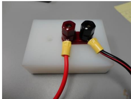
Figure 1: NBL Banana Plug Recetacle (electrical power)
